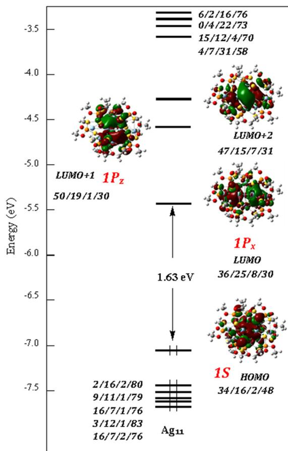
**Fig. 6** The Kohn–Sham orbital diagram of  $\text{Ag}_{11}$ . The orbital contribution (in %) is given in the order:  $(\text{Ag}_{\text{tbp}})_5/(\text{Ag}_{\text{cap}}^{\text{a,b}})_4/(\text{Ag}_{\text{ext}})_2/(\text{dtp})_8$ .
