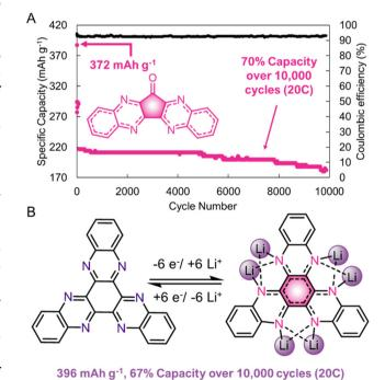
Fig. 9 (A). Performance of a quinoxaline-based cathode at a 20C rate.
