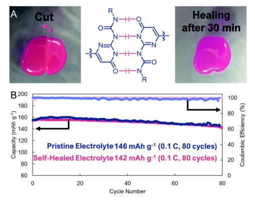
Fig. 10 (A). Optical images showing the self-healing process of the ureidopurimidinone-based electrolyte. (Left) The sample was cut into two pieces and (Right) after 30 minutes at 60 °C self-healing was observed. (B). Cycling stability comparing a cell containing pristine electrolyte, and electrolyte that has been cut, and then self-healed. Adapted with permissions from ref. 57. Copyright © 2018 Royal Society of Chemistry.
