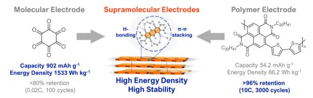
Fig. 2 Comparison of molecular and polymeric electrodes and their desirable features, which can be mutually accessed using supramolecular designs. Data for representative molecular, polymeric, and supramolecular electrodes were selected from ref. 18, 19 and 20, respectively.
