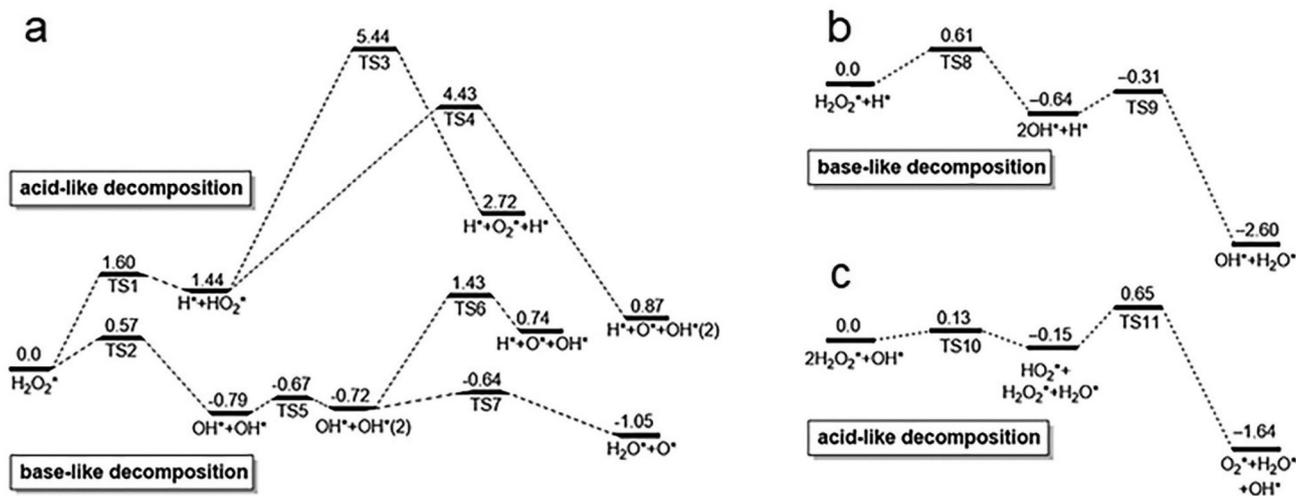
Fig. 6 Calculated reaction energy profiles for H<sub>2</sub>O<sub>2</sub> decomposition on the Au (111) surface under (a) neutral, (b) acidic, and (c) basic conditions. TS1–11 represent the intermediate states of H<sub>2</sub>O<sub>2</sub> adsorption and decomposition under different conditions, respectively. Reproduced from ref. 80 with permission from Elsevier Sci Ltd, copyright 2015.
