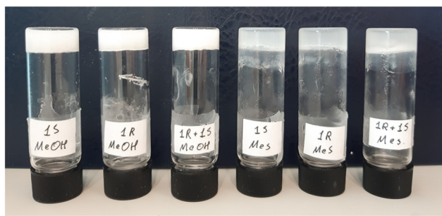
Fig. 1 Gels of 1S , 1R and 1R + 1S obtained from methanol (left) and mesitylene (right) at 2.0 wt/v%, respectively.
