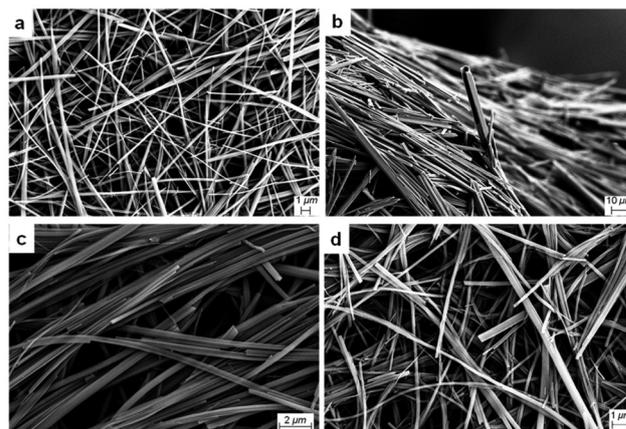
Fig. 3 SEM images of mixed MVBTA xerogels (2.0 wt/v%) in (a) methanol, (b) DMF/water (1 : 1, v/v), (c) mesitylene and (d) *o*-xylene.
