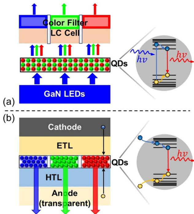
**Fig. 11** (a) The simplified structure of PL mode commercialised QLED TVs and their emission mechanism. (b) Structure of EL mode QLEDs and their emission mechanism. PERMISSION.<sup>129</sup>
