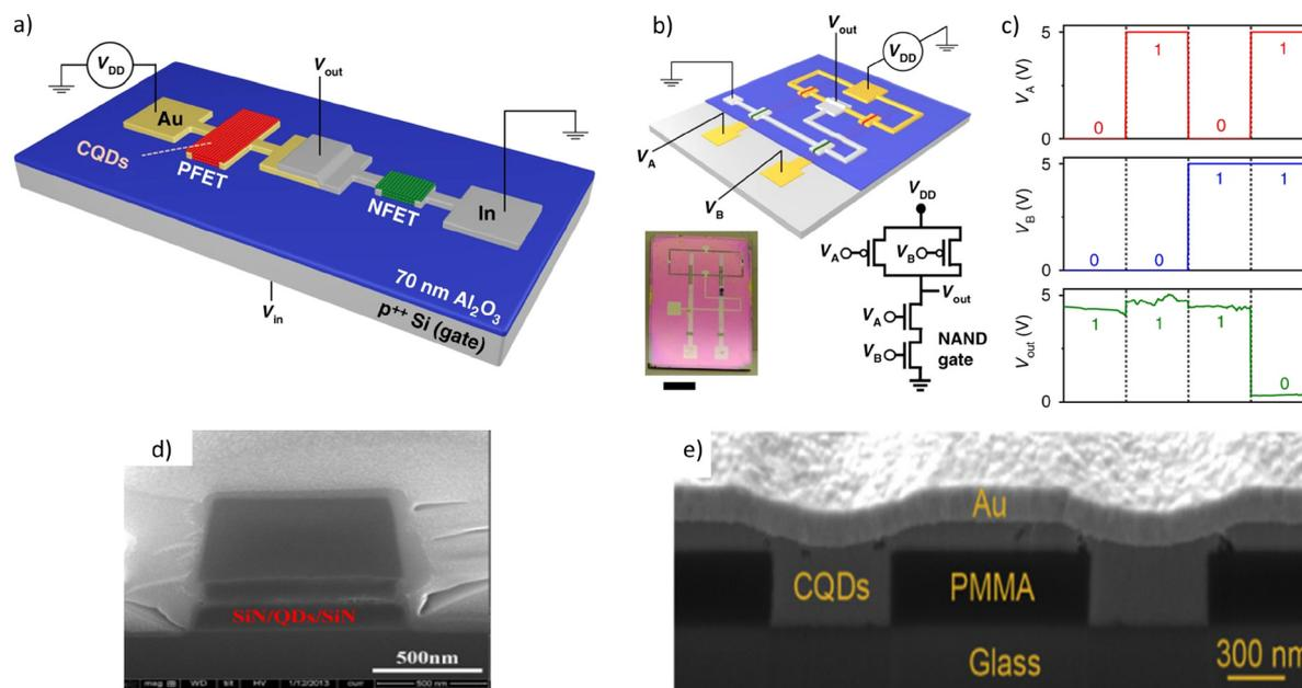
**Fig. 14** (a) The schematic structure of a CQD CMOS inverter, (b) a schematic illustration (top), its picture (bottom left) and the circuit diagram (bottom right) of a NAND gate made from the p and n-type CQD FETs and (c) the outcomes of the NAND gate for four different input configurations.<sup>88</sup> (d) Cross-sectional SEM image of the H-SiN/CQDs/L-SiN waveguide.<sup>156</sup> (e) Cross-sectional SEM image of a Y-splitter made from CQDs and PMMA.<sup>158</sup>
