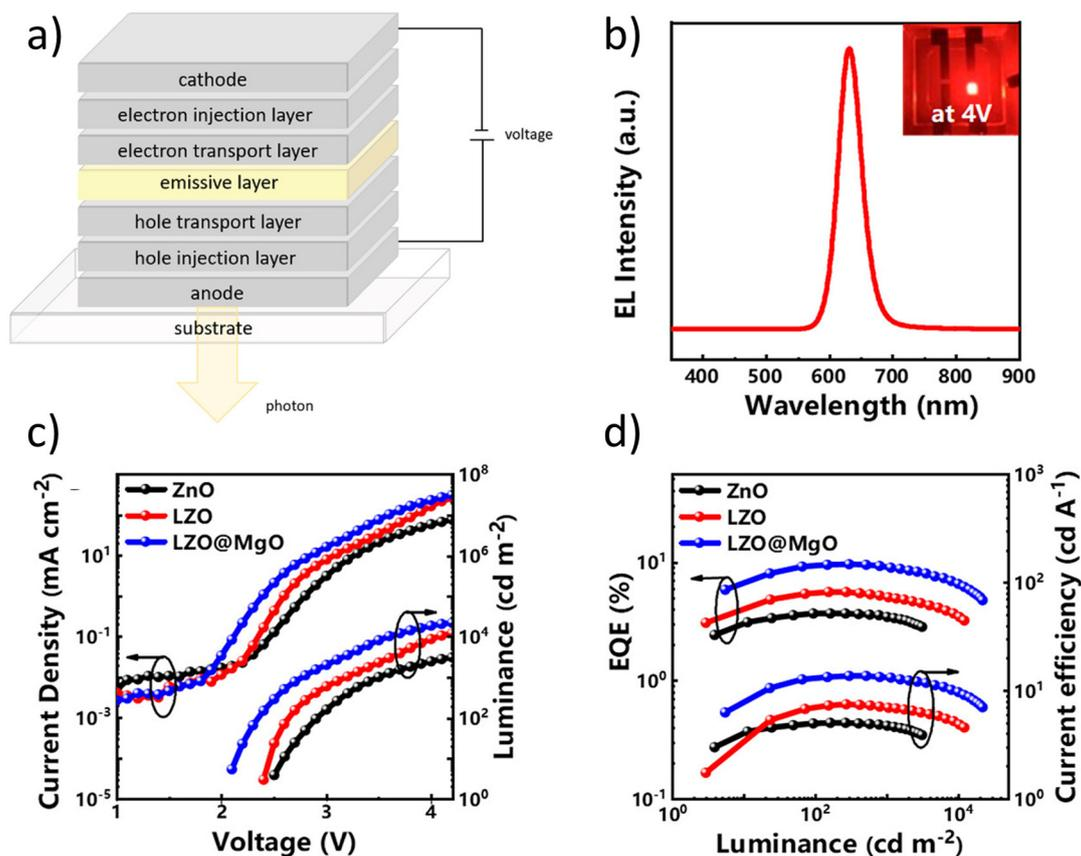
**Fig. 10** (a) The general structure of QLEDs. (b) The EL spectra and the (c) CD–V–L and (d) EQE–L–CE graphs of an InP-based QLED with different ETLs.<sup>121</sup>
