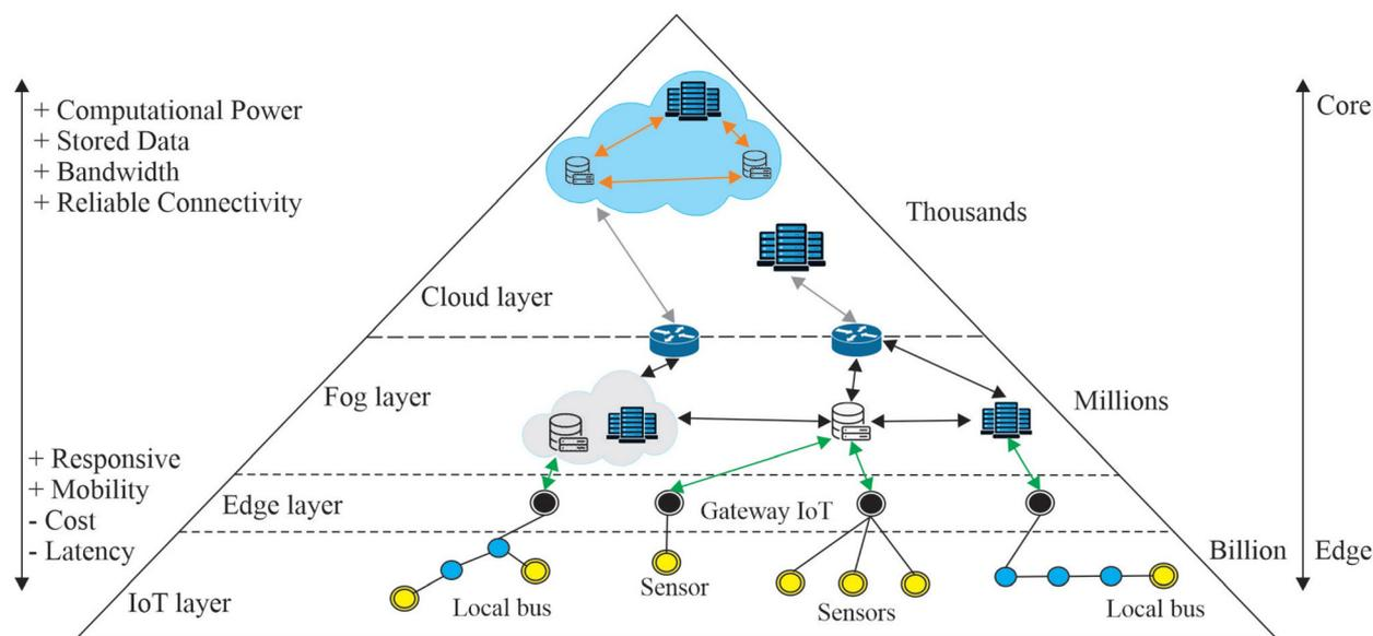
Fig. 5 Showing the different layers of the network, starting from the central cloud layer out into the edge and IoT layers. PERMISSION.<sup>56</sup>
