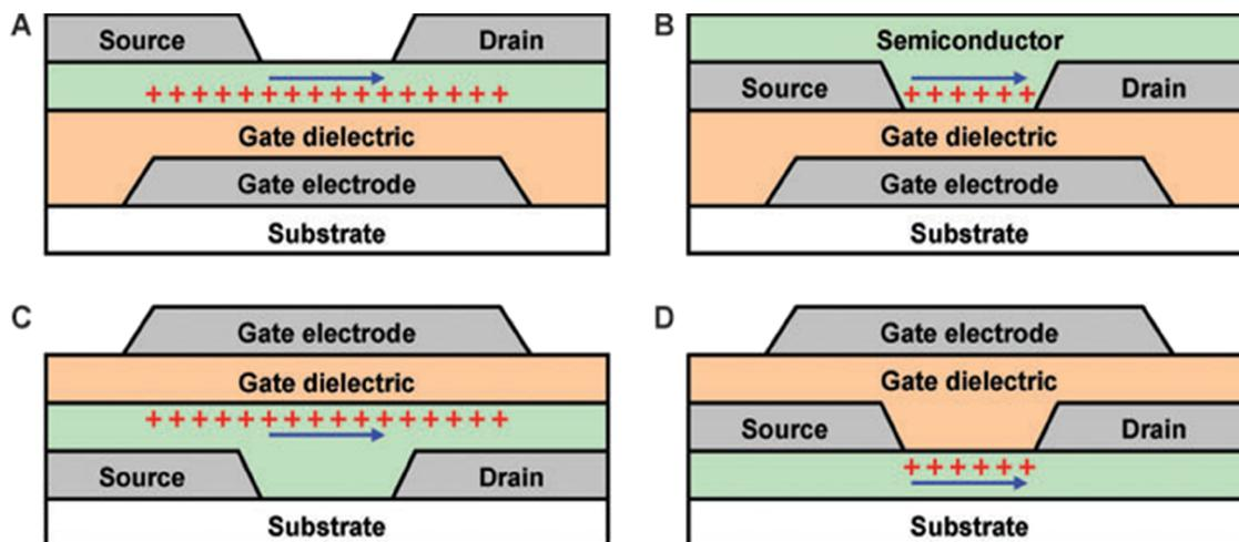
Fig. 6 Different structures of a TFT. (a) Bottom-gate staggered. (b) Bottom-gate coplanar. (c) Top-gate staggered. (d) Top-gate coplanar.<sup>68</sup>
