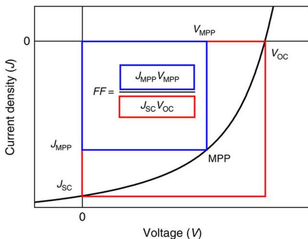
**Fig. 13** Current density-voltage graph for a photovoltaic cell, showing the positions of important parameters.<sup>148</sup>
