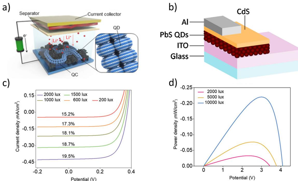
**Fig. 12** (a) Schematic structure of a CQD quantum chain incorporated into lithium-ion battery.<sup>138</sup> (b) Structure of a typical CQD solar cell.<sup>139</sup> (c)  $J$ - $V$  Curves at different irradiances and their respective PCE values and (d) power density- $V$  curves at different irradiances for a PbS-based photovoltaic cell.<sup>140</sup>
