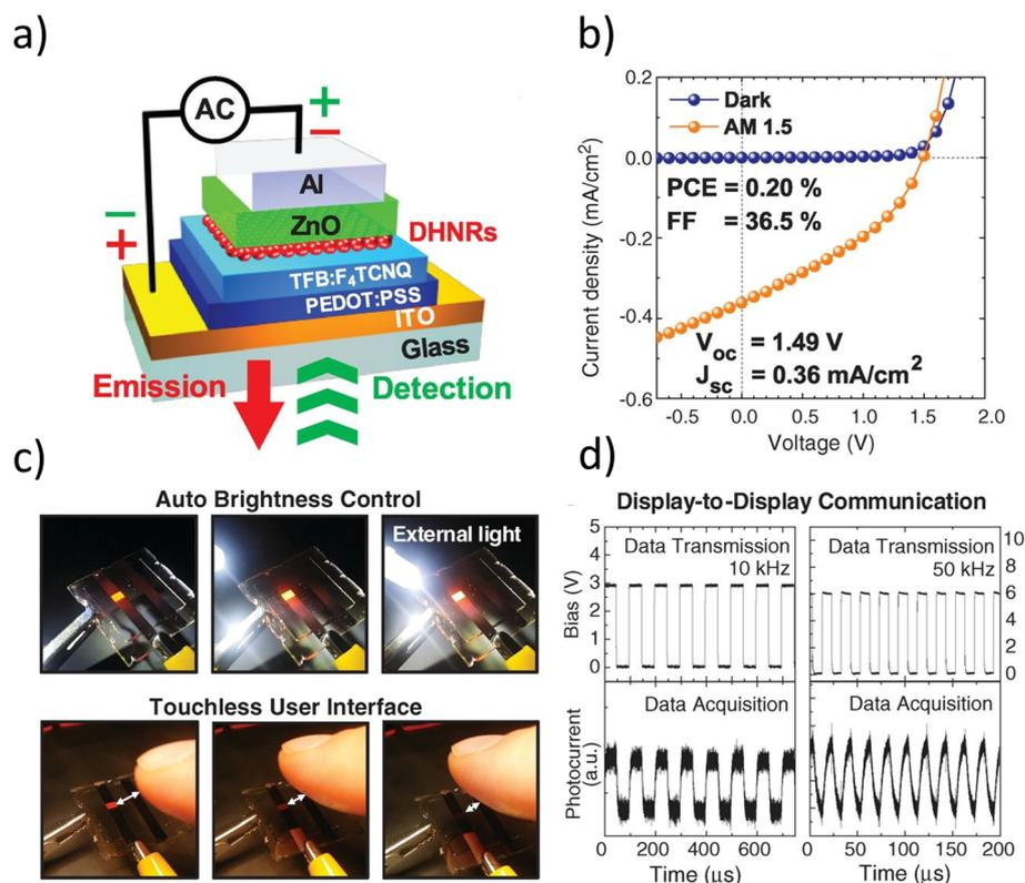
**Fig. 16** (a) Structure of the dual-function DHNR device. (b) The *J-V* characteristics of the device under Dark and AM 1.5 (100 mW cm<sup>-2</sup> conditions). (c) The automatic brightness control in response to an LED and finger approaching the device. (d) Data transmission and acquisition between two identical devices at 10 and 50 kHz.<sup>175</sup>
