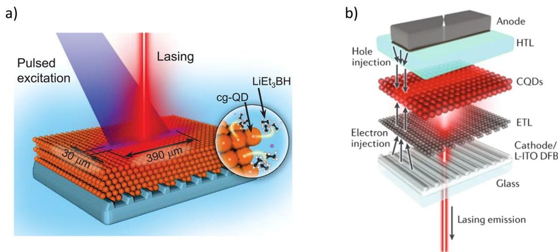
Fig. 15 Structure of (a) an optically pumped CQD laser operating via a DFB structure<sup>168</sup> and (b) a potential electrically pumped CQD laser, demonstrated to work by pumping optically.<sup>169</sup>
