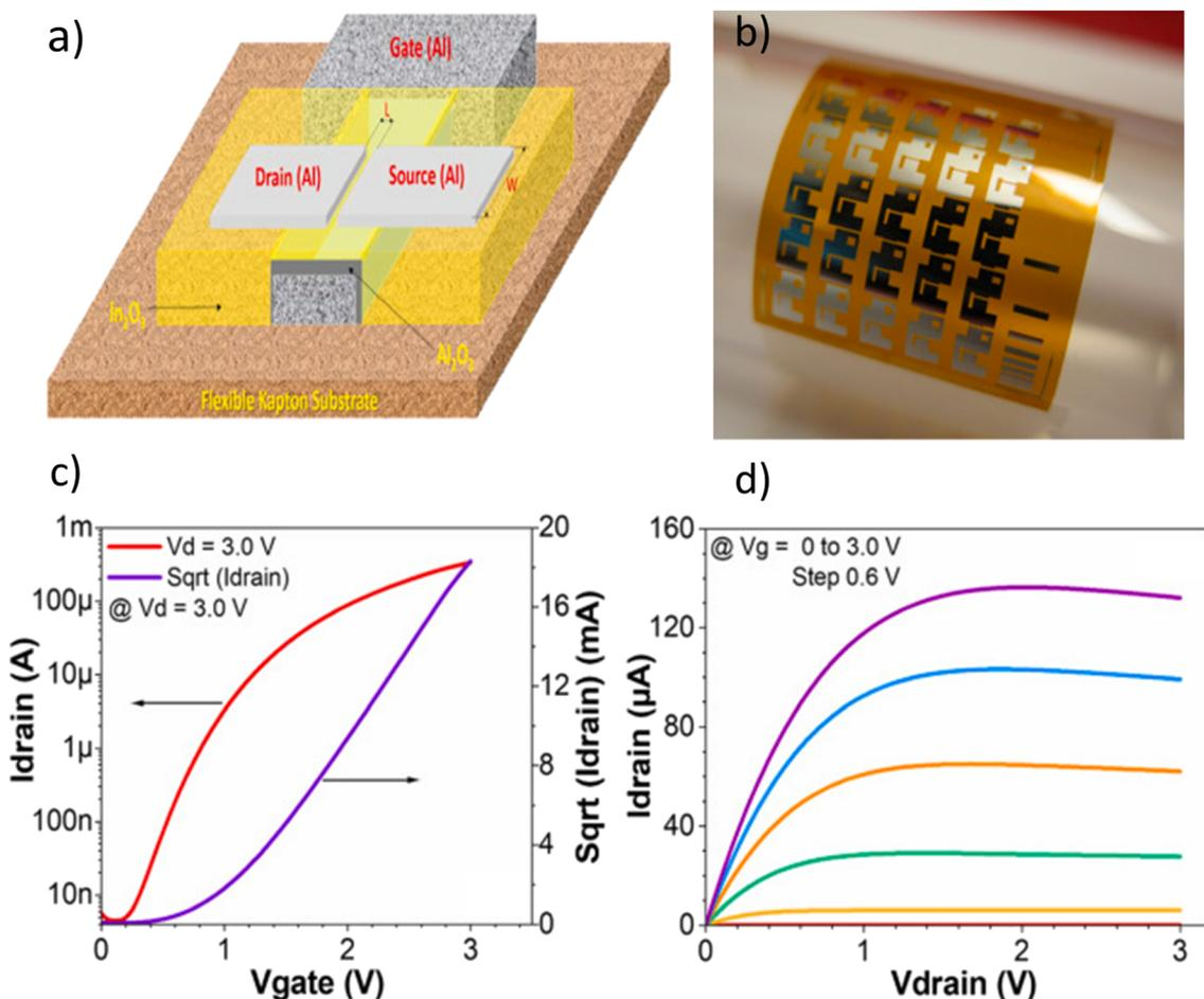
Fig. 7 (a) The structure of an  $\text{In}_2\text{O}_3$  flexible TFT on a flexible substrate. (b) A camera image of the TFTs. The (c)  $I_D$ - $V_G$  and (d)  $I_D$ - $V_D$  graphs of the TFTs.<sup>76</sup>
