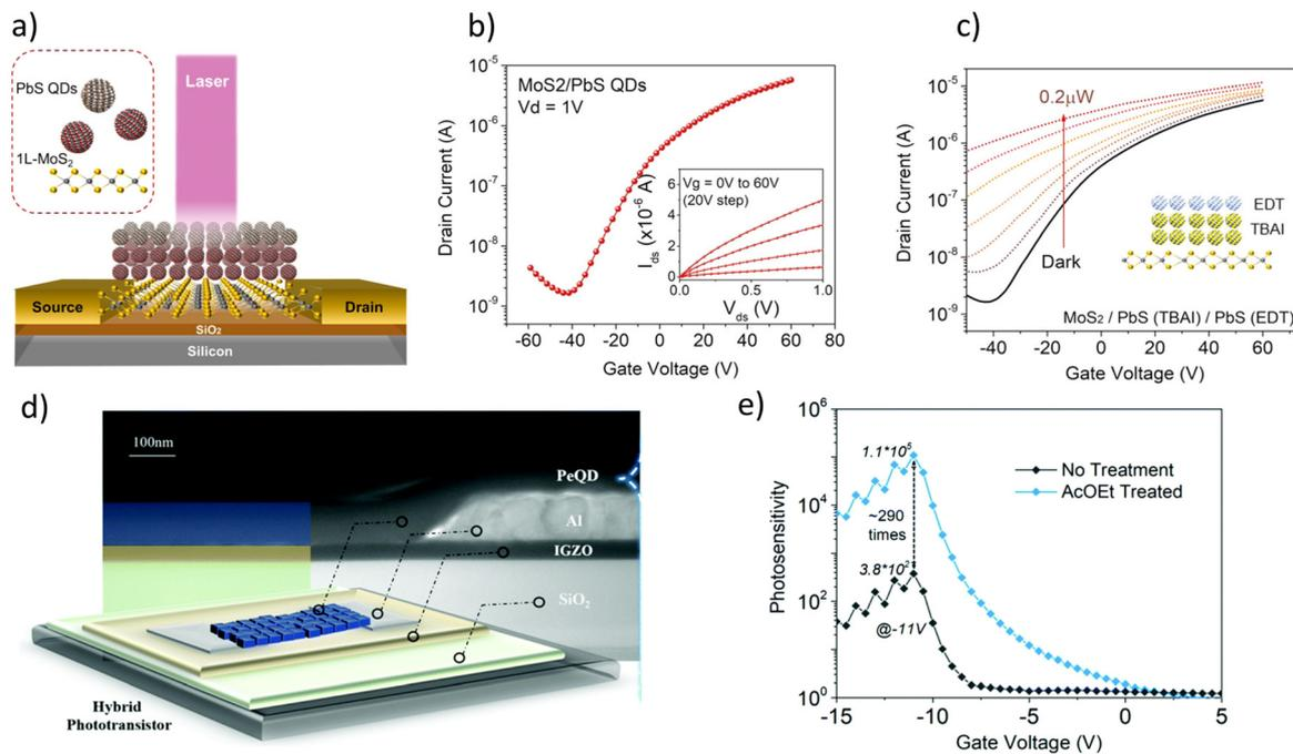
**Fig. 9** (a) The structure of a PbS/MoS<sub>2</sub> phototransistor, its respective (b)  $I_D$ - $V_G$  graph (inset:  $I_D$ - $V_D$  for different  $V_G$ ) and (c)  $I_D$ - $V_G$  graph at different illumination powers.<sup>95</sup> (d) The structure of hybrid perovskite QD and its (e) PR- $V_{GS}$  graph.<sup>94</sup>
