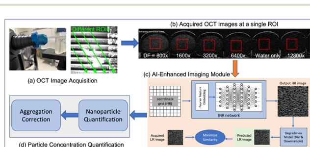
Fig. 1 AI-enhanced OCT imaging for nanoparticle quantification.
