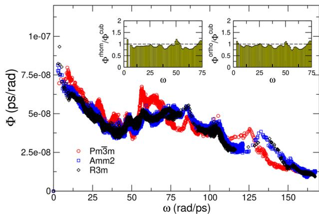
**Fig. 5** Phase space of three-phonon processes allowed by the conservation of energy and momentum in KNO. Results are expressed as a function of phonon frequency and the insets show the phase space ratio for the polar and nonpolar phases considered in this study.
