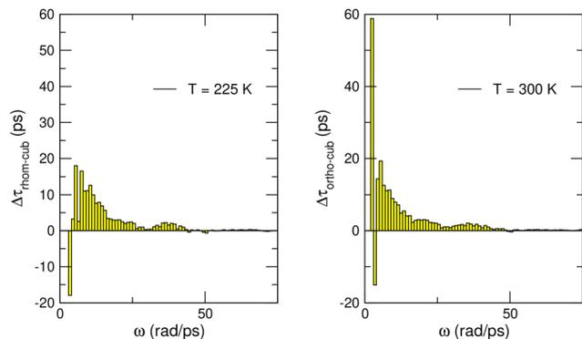
**Fig. 6** Phonon lifetimes of the polar and nonpolar phases of KNO expressed as a function of phonon frequency.  $\Delta\tau_{x\text{-cub}} \equiv \tau_x - \tau_{\text{cub}}$  results are averaged over frequency intervals of  $1 \text{ rad ps}^{-1}$  and correspond to  $R3m \rightarrow Pm\bar{3}m$  at 225 K and  $Amm2 \rightarrow Pm\bar{3}m$  at 300 K.
