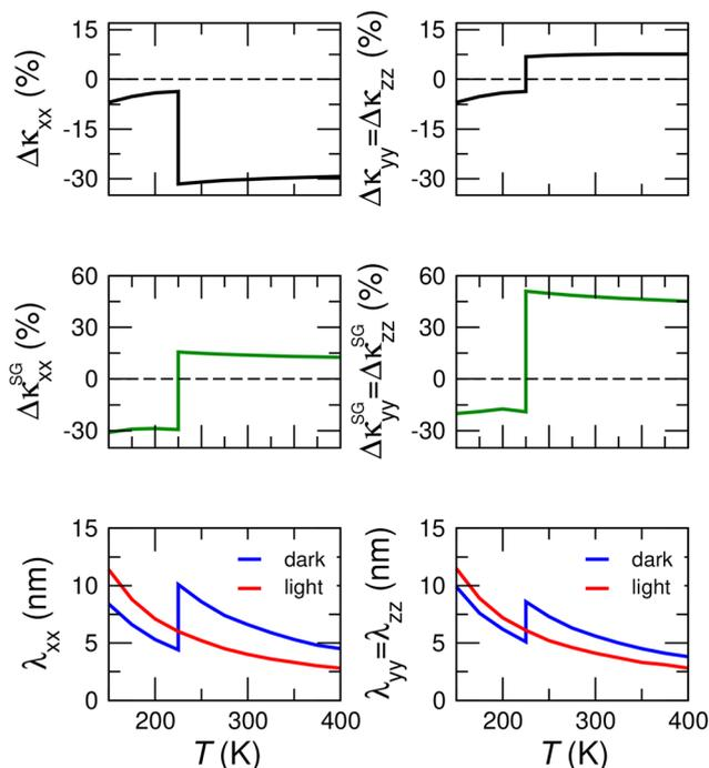
**Fig. 4** Thermal conductivity variations in KNO upon the light-induced polar  $\rightarrow$  nonpolar phase transformation. (Top) Directly deduced from Fig. 3. (Middle) Considering a uniform phonon mean free path of 1 nm (small-grain approximation). (Bottom) Effective global phonon mean free path,  $\lambda$ , computed as  $\kappa/\kappa^{\text{SG}}$ .
