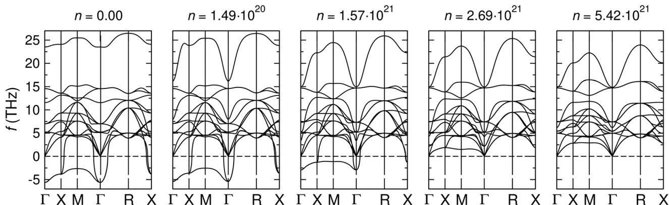
**Fig. 2** Phonon dispersion of KNO in the nonpolar cubic phase for different photoexcited carrier densities. Photoexcited carrier densities were obtained by smearing the Fermi distribution with widths equal to 0.01, 0.10, 0.30, 0.50, and 0.70 eV (left to right);  $n$  is expressed in units of conduction electrons per  $\text{cm}^3$ .
