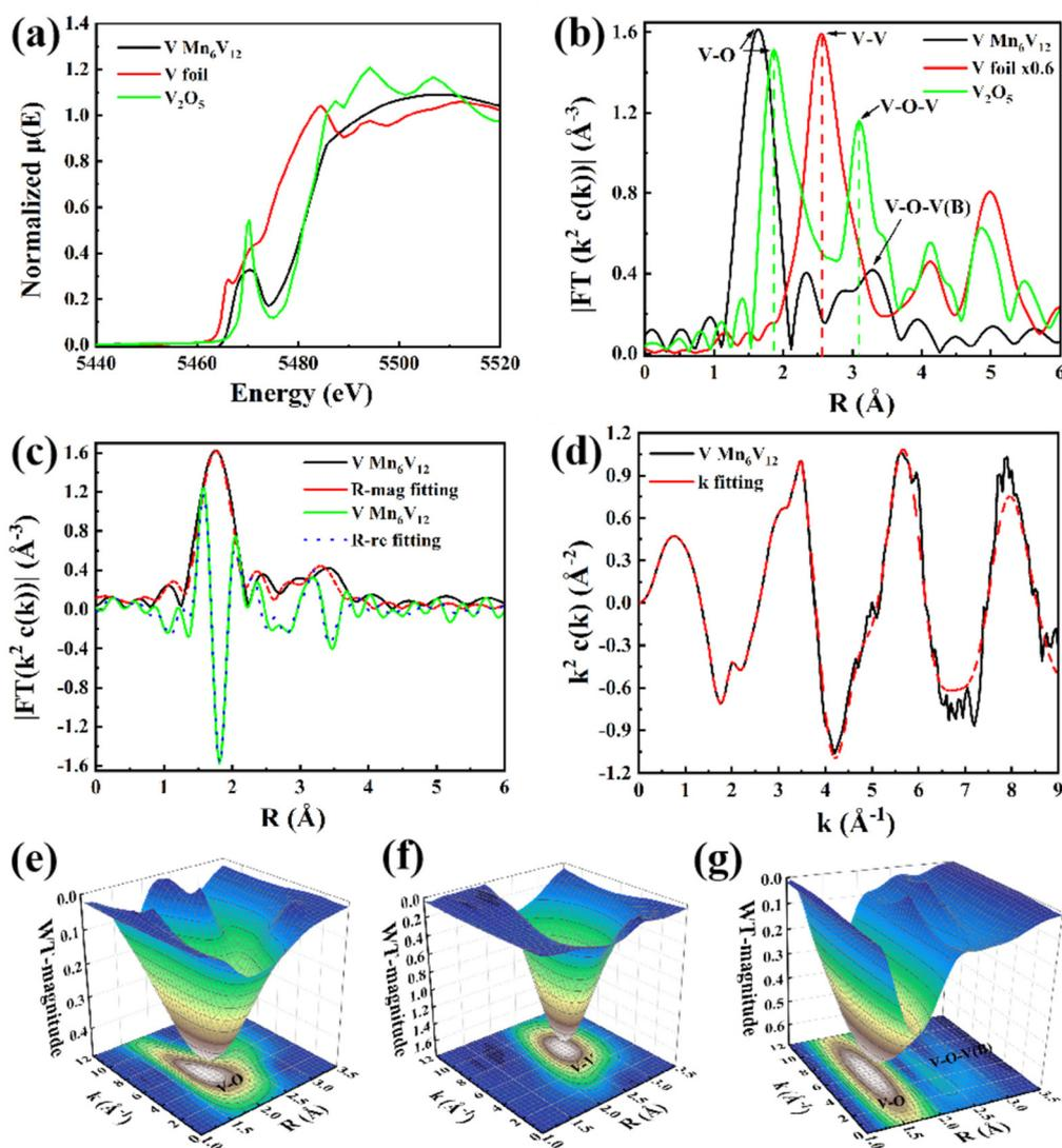
**Fig. 2** (a) V K-edge normalized XANES spectra, (b) FT curves of V K-edge EXAFS spectra, (c) V K-edge EXAFS curve fitting at  $R$  space and  $q$  space, (d) V K-edge EXAFS curve fitting at  $k$  space, (e) wavelet transform EXAFS of  $V_2O_5$ , (f) Wavelet transform EXAFS of V foil, (g) wavelet transform EXAFS of  $Mn_6V_{12}$ .
