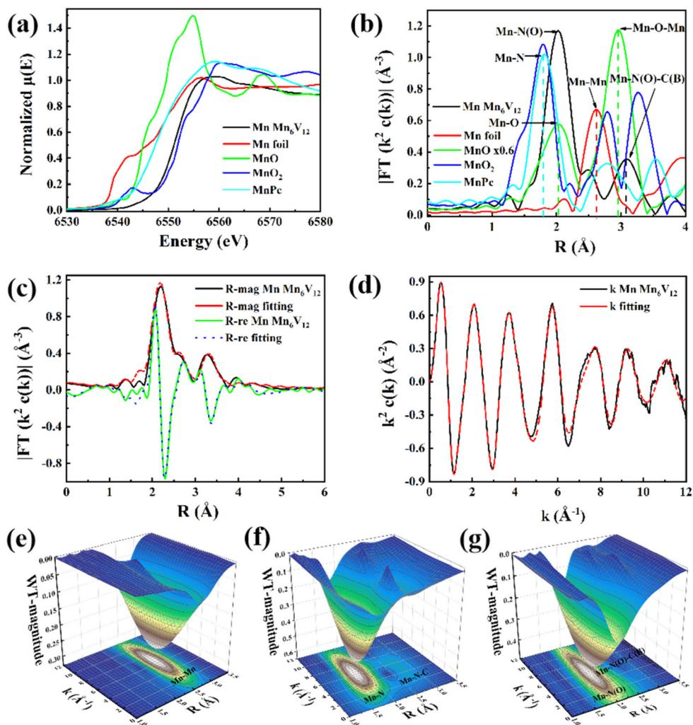
Fig. 3 (a) Mn K-edge normalized XANES spectra, (b) FT curves of Mn K-edge EXAFS spectra, (c) Mn K-edge EXAFS curve fitting at  $R$  space and  $q$  space, (d) Mn K-edge EXAFS curve fitting at  $k$  space, (e) wavelet transform EXAFS of Mn foil, (f) wavelet transform EXAFS of MnPC, (g) wavelet transform EXAFS of  $\text{Mn}_6\text{V}_{12}$ .
