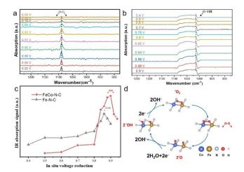
**Fig. 6** In situ FTIR characterization of (a) FeCo–N–C and (b) Fe–N–C. (c) FTIR absorption stretching at 1090 cm<sup>-1</sup> for FeCo–N–C and 1014 cm<sup>-1</sup> for Fe–N–C. (d) Schematic of the ORR mechanism for FeCo–N–C.
