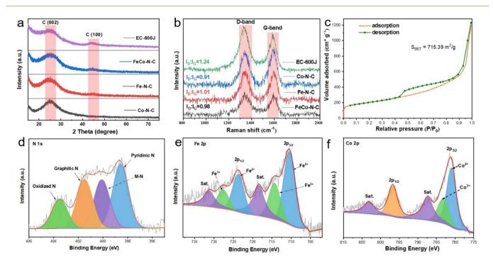
Fig. 2 (a) XRD patterns and (b) Raman spectra of FeCo-N-C. (c) N<sub>2</sub> adsorption-desorption isotherm curve and pore size distribution of FeCo-N-C. (d) N 1s, (e) Fe 2p and (f) Co 2p XPS spectra of FeCo-N-C.
