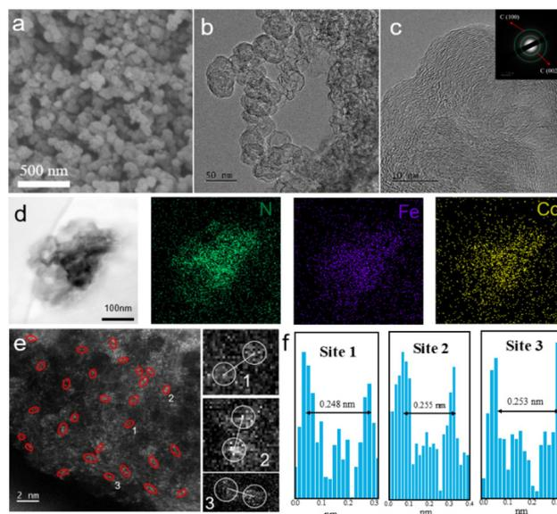
**Fig. 1** (a) SEM image of FeCo-N-C. (b and c) TEM and SAED (inset) images of FeCo-N-C. (d) HAADF-STEM and the corresponding elemental mapping images of FeCo-N-C. (e) Aberration-corrected HAADF-STEM image of FeCo-N-C, where some Fe-Co diatomic sites are highlighted by red circles (the red circles 1, 2 and 3 are partially enlarged on the right). (f) Intensity profiles of the three numbered sites in (e).
