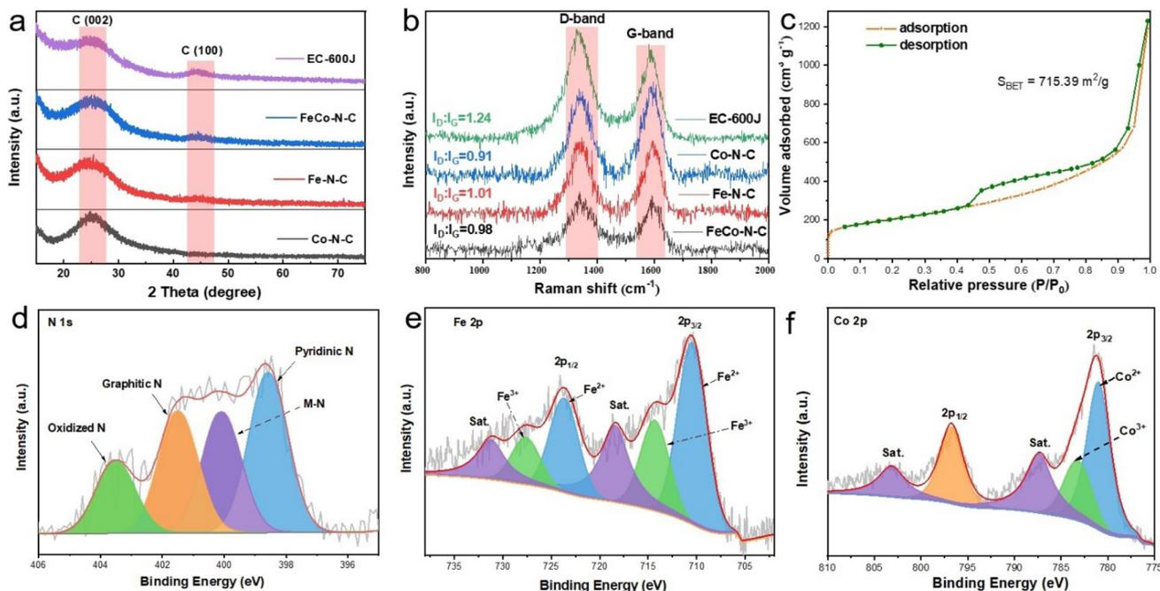
Fig. 2 (a) XRD patterns and (b) Raman spectra of FeCo-N-C. (c)  $\text{N}_2$  adsorption-desorption isotherm curve and pore size distribution of FeCo-N-C. (d) N 1s, (e) Fe 2p and (f) Co 2p XPS spectra of FeCo-N-C.
