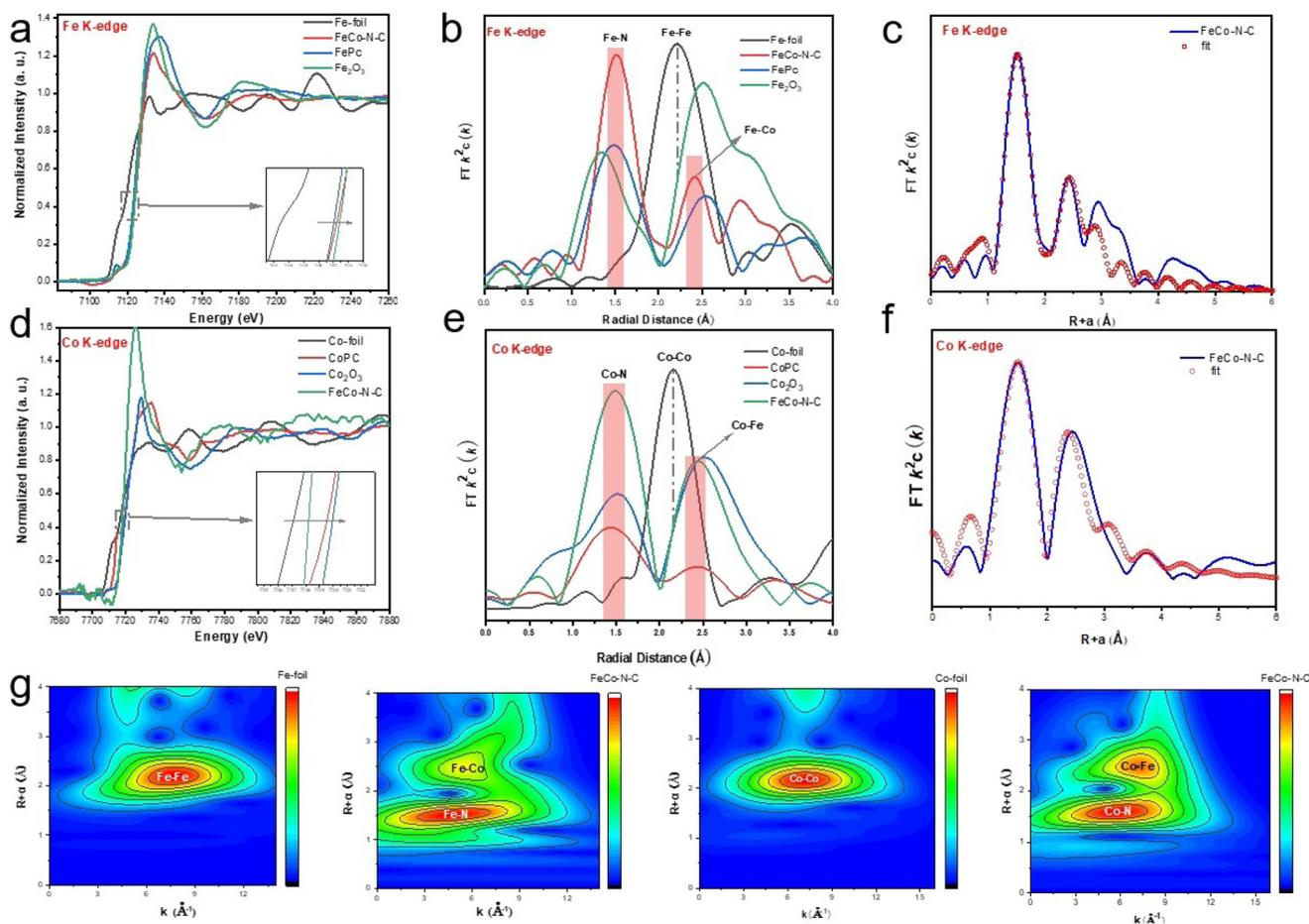
**Fig. 3** (a) Fe K-edge XANES spectra of FeCo–N–C,  $Fe_2O_3$ , FePc and Fe foil. (b) Fourier transform EXAFS spectra at the R-space of Fe. (d) Co K-edge XANES spectra of FeCo–N–C,  $Co_2O_3$ , CoPc and Co foil. (e) Fourier transform EXAFS spectra at the R-space of Co. Fitting curves in the R-space for (c) Fe and (f) Co. (g) WT  $k^3$ -weighted EXAFS spectra and the corresponding metal foil reference.
