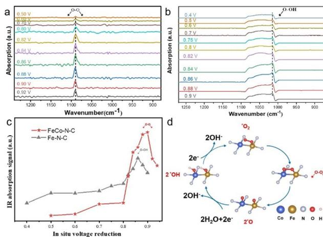
**Fig. 6** *In situ* FTIR characterization of (a) FeCo-N-C and (b) Fe-N-C. (c) FTIR absorption stretching at  $1090 \text{ cm}^{-1}$  for FeCo-N-C and  $1014 \text{ cm}^{-1}$  for Fe-N-C. (d) Schematic of the ORR mechanism for FeCo-N-C.
