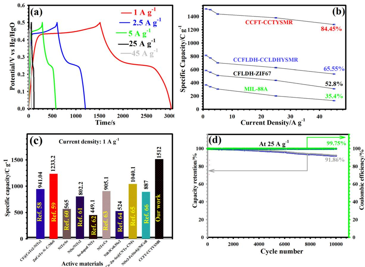
**Fig. 5** (a) GCD graphs of the CCFT–CCTYSMR from 1 to 45 A g<sup>-1</sup> (GCD tests were repeated three times). (b) Specific capacities vs. current densities of the CCFT–CCTYSMR, CCFLDH–CCLDHYSMR, CFLDH–ZIF67, and MIL-88A electrodes with the error bar. (c) Comparison of capacity of the CCFT–CCTYSMR at 1 A g<sup>-1</sup> with the previous literature. (d) Longevity and coulombic efficiency of the CCFT–CCTYSMR at 25 A g<sup>-1</sup>.
