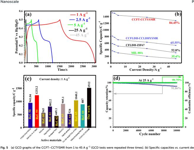
Fig. 5 (a) GCD graphs of the CCFT-CCTYSMR from 1 to 45 A g<sup>-1</sup> (GCD tests were repeated three times). (b) Specific capacities vs. current densities of the CCFT-CCTYSMR, CCFLDH-CCLDHYSMR, CFLDH-ZIF67, and MIL-88A electrodes with the error bar. (c) Comparison of capacity of the CCFT-CCTYSMR at 1 A  $g^{-1}$  with the previous literature. (d) Longevity and coulombic efficiency of the CCFT-CCTYSMR at 25 A  $g^{-1}$ .
