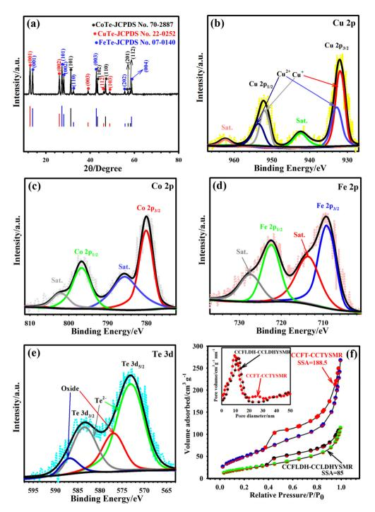
Fig. 3 (a) XRD of the CCFT–CCTYSMR. (b) Cu 2p XPS pattern of the CCFT–CCTYSMR. (c) Co 2p XPS pattern of the CCFT–CCTYSMR. (d) Fe 2p XPS pattern of the CCFT–CCTYSMR. (e) Te 3d XPS pattern of the CCFT–CCTYSMR. (f) BET curves of the CCFT–CCTYSMR and CCFLDH–CCLDHYSMR and their corresponding BJH curves (inset).
