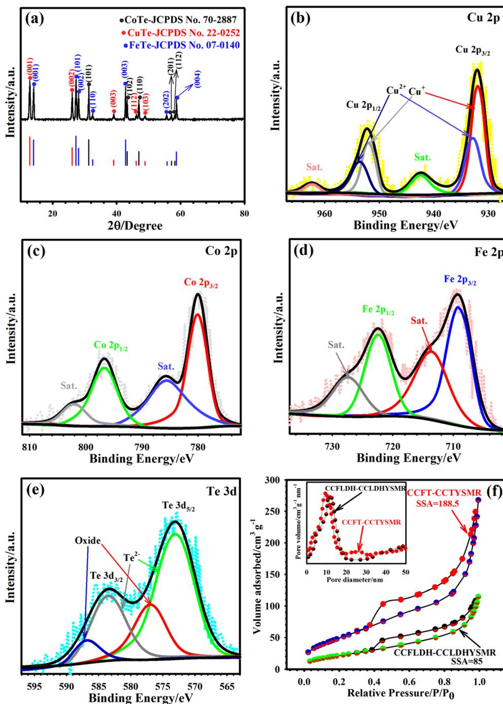
**Fig. 3** (a) XRD of the CCFT-CCTYSMR. (b) Cu 2p XPS pattern of the CCFT-CCTYSMR. (c) Co 2p XPS pattern of the CCFT-CCTYSMR. (d) Fe 2p XPS pattern of the CCFT-CCTYSMR. (e) Te 3d XPS pattern of the CCFT-CCTYSMR. (f) BET curves of the CCFT-CCTYSMR and CCFLDH-CCLDHYSMR and their corresponding BJH curves (inset).
