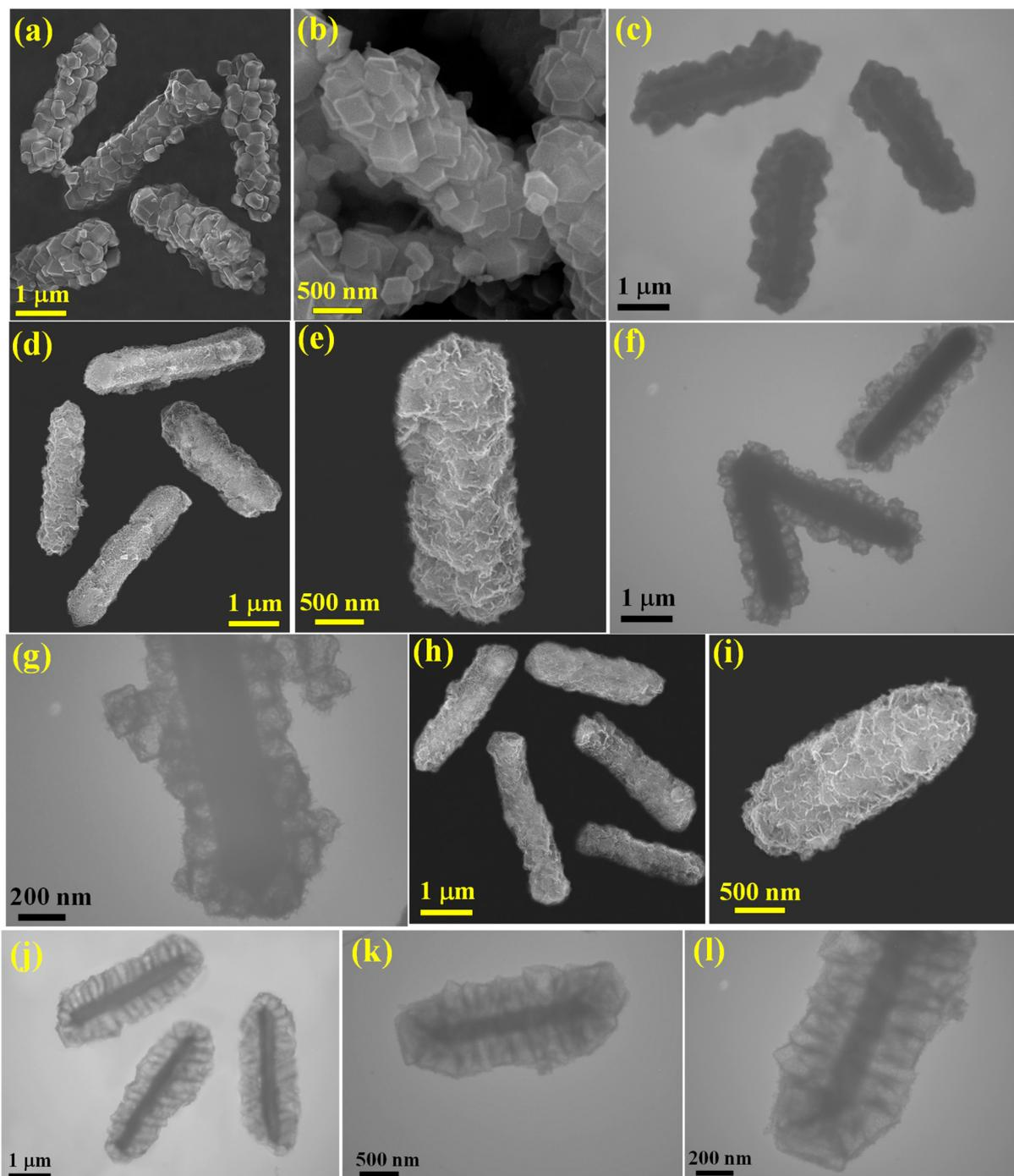
**Fig. 2** (a and b) FESEM images of the CFLDH–ZIF67. (c) TEM image of the CFLDH–ZIF67. (d and e) FESEM images of the CCFLDH–CCLDHYSMR. (f and g) TEM images of the CCFLDH–CCLDHYSMR. (h and i) FESEM images of the CCFT–CCTYSMR. (j–l) TEM images of the CCFT–CCTYSMR.
