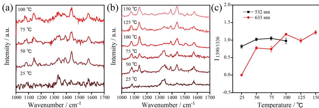
**Fig. 5** Temperature-dependent SERS spectra of the plasmon-induced photocatalytic reaction of 4-NTP at high temperatures with 532 nm (a) and 633 nm (b) excitation, respectively,  $t_{\text{acq}} = 60$  s. (c) intensity ratio of  $1390\text{ cm}^{-1}/1336\text{ cm}^{-1}$  referring to [DMAB]/[4-NTP] as a function of temperature at 532 nm (black) and 633 nm (red) ( $P_{532\text{ nm}} = 1.05\text{ }\mu\text{W}$ ,  $P_{633\text{ nm}} = 7.8\text{ }\mu\text{W}$ ).
