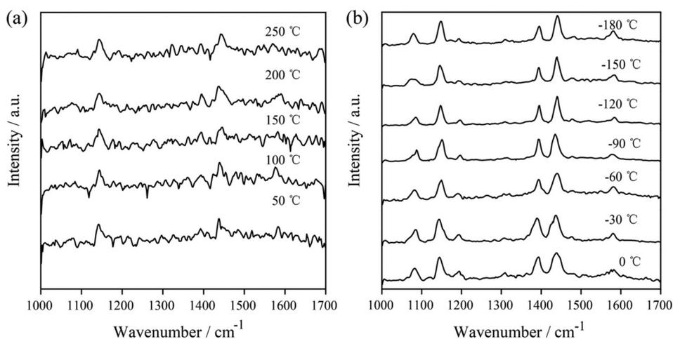
**Fig. 6** Temperature-dependent SERS spectra of the plasmon-induced photocatalytic reaction of 4-ATP at 50–250 °C (a) and at –180–0 °C (b) with 532 nm excitation ( $P = 1.05\text{ }\mu\text{W}$ ,  $t_{\text{acq}} = 60$  s).
