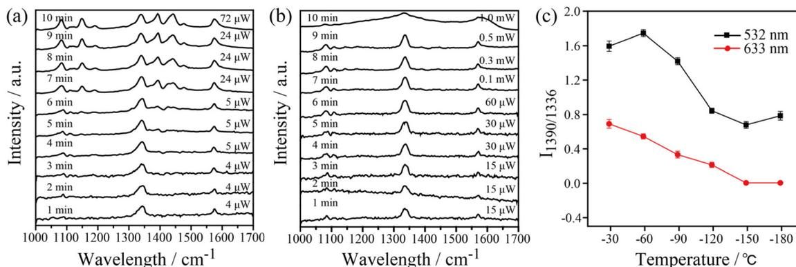
Fig. 4 Time-dependent SERS spectra of the plasmon-induced catalytic reaction of 4-NTP at  $-180\text{ }^{\circ}\text{C}$  with (a) 532 nm and (b) 633 nm excitation at different laser powers on the samples. The time interval is 1 min from bottom to top,  $t_{\text{acq}} = 60\text{ s}$ ; (c) the average intensity ratio of 1390  $\text{cm}^{-1}$ /1336  $\text{cm}^{-1}$  referring to [DMAB]/[4-NTP] as a function of temperature at 532 nm (black) and 633 nm (red).
