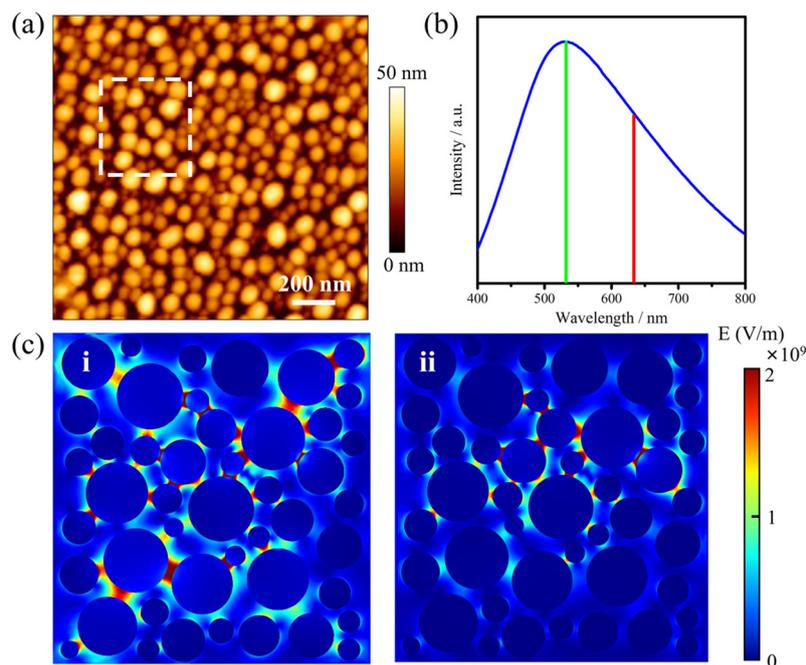
Fig. 2 (a) AFM topography image and (b) normalized extinction spectrum of AgNIs; (c) simulated electric field distribution of AgNIs (a  $300 \times 300 \text{ nm}^2$  region extracted from the AFM image) under 532 nm (i) and 633 nm (ii) excitation, respectively.
