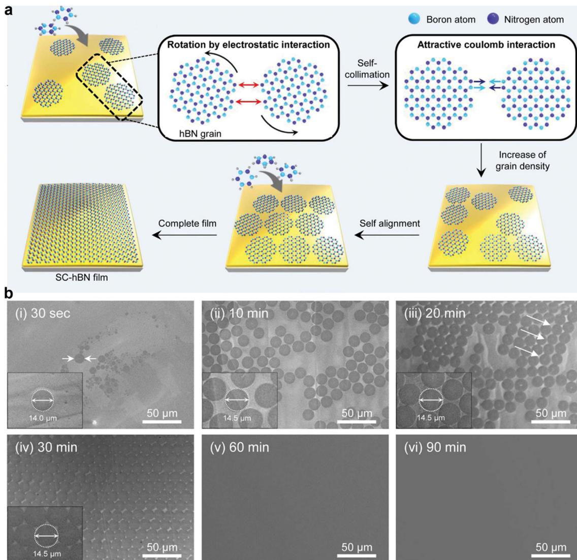
**Fig. 6** (a) Schematic illustration of the synthesis of the wafer-scale single crystal hexagonal boron nitride (hBN) film *via* self-collimation of randomly oriented grains on a liquid Au surface. (b) Scanning electron microscopy images of the hBN thin film growth process at different growth times. [Fig. 6 is reproduced with permission from Lee *et al.*<sup>20</sup> Copyright 2018, American Association for the Advancement of Science].
