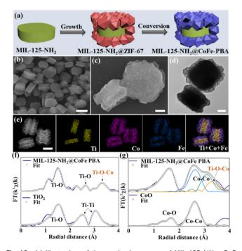
Fig. 10 (a) Illustration of the synthesis process of MIL-125-NH<sub>2</sub>@CoFe PBA. (b and c) SEM, (d) TEM, (e) HAADF-STEM and the corresponding elemental mapping images. Scale bars are: (b), 1 µm; (e), 500 nm; and (c and d), 200 nm. (f) Ti coordination environments of MIL-125-NH<sub>2</sub>@CoFe PBA and TiO<sub>2</sub> and (g) Co coordination environments of MIL-125-NH<sub>2</sub>@CoFe PBA and CoO. Reprinted with permission from ref. 44. Copyright 2023 Wiley-VCH.
