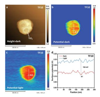
**Fig. 4** (a) AFM and (b) KPFM images of TF in the absence of light. (c) KPFM image of TF under UV light illumination at 365 nm. (d) Corresponding surface potential profiles. Reprinted with permission from ref. 69. Copyright 2022 Wiley-VCH.
