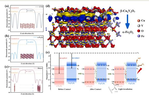
Fig. 5 Work functions of (a) CVO (010), (b)  $\alpha$ -Fe<sub>2</sub>O<sub>3</sub> (001), and (c) heterojunctions. (d) Charge density difference at the CVO (010)/ $\alpha$ -Fe<sub>2</sub>O<sub>3</sub> (001) interface, yellow indicates the loss of electrons and blue represents the gain of electrons. (e) Photocatalytic mechanism of S-scheme heterojunctions. Reprinted with permission from ref. 75. Copyright 2023 Elsevier.
