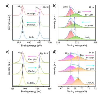
Fig. 3 High-resolution XPS spectra of (a) Sn 3d, (b) O 1s, (c) Bi 4f, and (d) Br 3d for  $SnO_2$ ,  $Cs_3Bi_2Br_9$ , and SC4 obtained in the dark and under UV light irradiation, respectively. Reprinted with permission from ref. 66. Copyright 2023 American Chemical Society.
