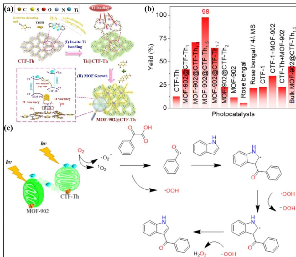
**Fig. 14** (a) Schematic presentation of the synthetic route of the MOF-902@CTF-Th heterostructure. (b) Decarboxylative C3-acylation of indoles of different photocatalysts. (c) Proposed reaction mechanism for decarboxylative C3-acylation of indoles in the presence of the MOF-902@CTF-Th photocatalyst. Reprinted with permission from ref. 46. Copyright 2023 Wiley-VCH.
