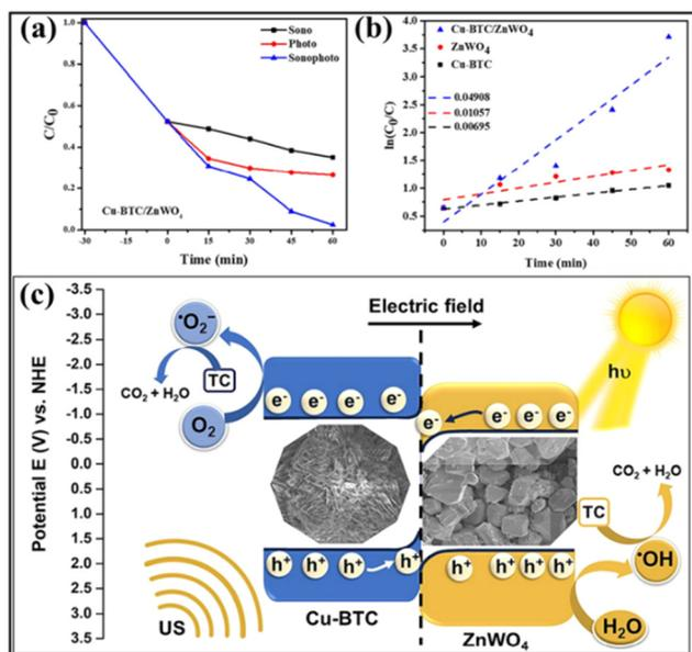
**Fig. 16** (a) Analysis of Cu-BTC/ZnWO<sub>4</sub> using C/C<sub>0</sub> plots for sono-, photo-, and sonophotocatalytic processes. (b) Kinetic studies of Cu-BTC, ZnWO<sub>4</sub>, and Cu-BTC/ZnWO<sub>4</sub>. (c) Schematic illustration depicting the degradation of TC using sonophotocatalysis on Cu-BTC/ZnWO<sub>4</sub> S-scheme photocatalysts. Reprinted with permission from ref. 138. Copyright 2023 Elsevier.
