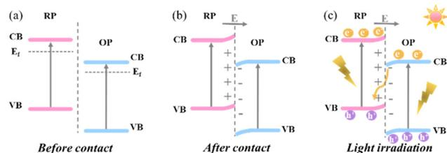
**Fig. 2** Graphical illustration of the charge migration process of S-scheme heterojunctions. (a) before contact; (b) after contact; and (c) photogenerated charge carrier transfer under light irradiation.
