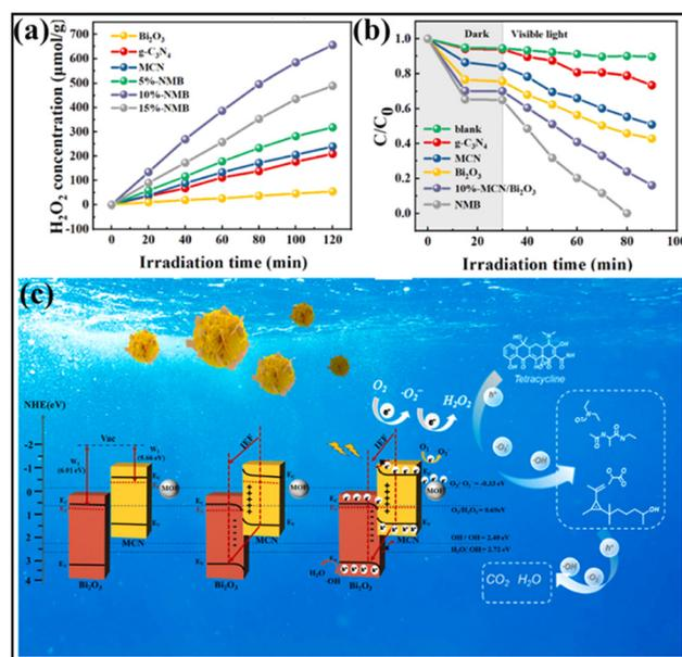
**Fig. 17** (a) Degradation performance of TC using various photocatalysts. (b) H<sub>2</sub>O<sub>2</sub> production performances of different photocatalysts. (c) Illustration of the proposed photocatalytic mechanism of 10%-NMB based on S-scheme charge transfer for the degradation of TC. Reprinted with permission from ref. 139. Copyright 2023 Elsevier.
