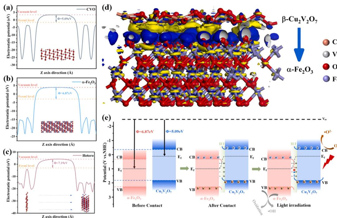
**Fig. 5** Work functions of (a) CVO (010), (b)  $\alpha\text{-Fe}_2\text{O}_3$  (001), and (c) heterojunctions. (d) Charge density difference at the CVO (010)/ $\alpha\text{-Fe}_2\text{O}_3$  (001) interface, yellow indicates the loss of electrons and blue represents the gain of electrons. (e) Photocatalytic mechanism of S-scheme heterojunctions. Reprinted with permission from ref. 75. Copyright 2023 Elsevier.
