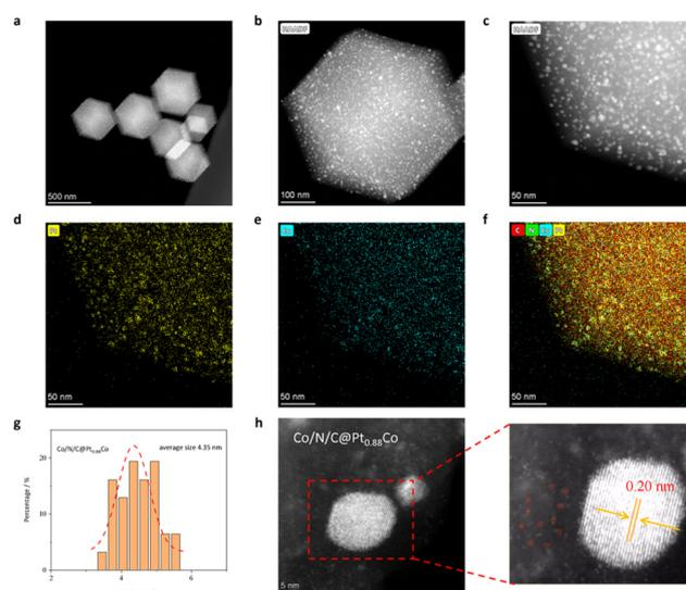
**Fig. 2** (a–c) HAADF-STEM images of Co/N/C@Pt<sub>0.88</sub>Co. (d–f) EDX images of Co/N/C@Pt<sub>0.88</sub>Co. (g) Size distribution of PtCo nanoparticles in the Co/N/C@Pt<sub>0.88</sub>Co catalyst. (h) The HAADF-STEM image of the hybrid catalyst and an individual nanoparticle in the Co/N/C@Pt<sub>0.88</sub>Co catalyst.
