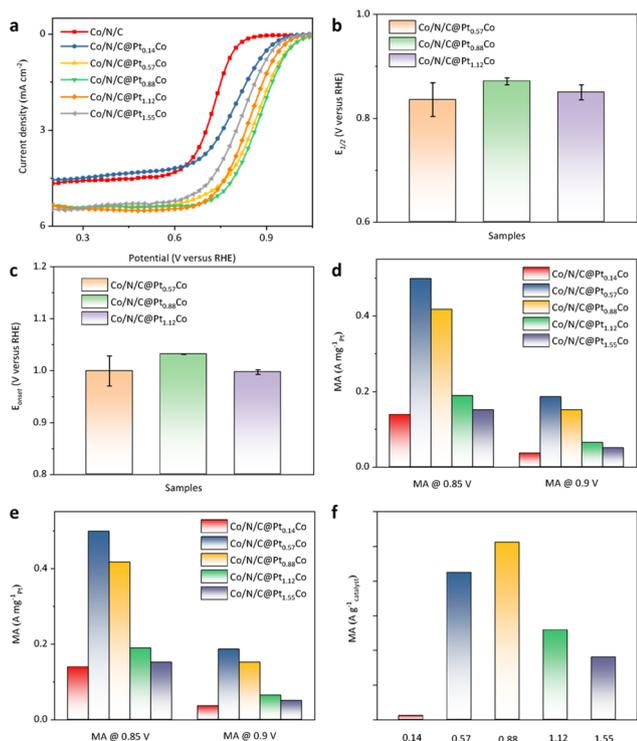
**Fig. 3** (a) ORR polarization curves, (b) onset potential ( $E_{\text{onset}}$ ), (c) half-wave potential ( $E_{1/2}$ ), (d) mass activity normalized to Pt mass, (e) mass activity normalized to catalyst mass and (f) the mass activity and Pt/Co ratio (horizontal axis) showing a volcanic-like curve.
