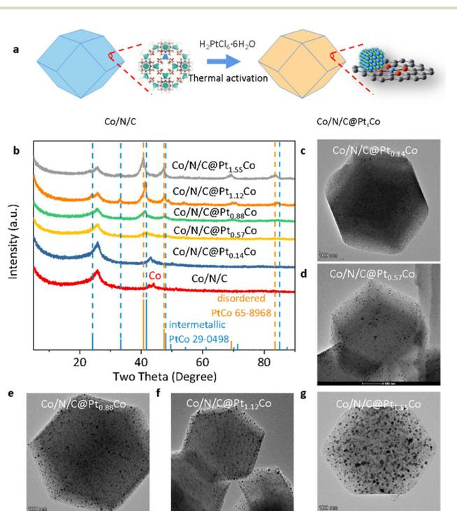
**Fig. 1** (a) Schematic of the synthesis of Co/N/C@Pt<sub>x</sub>Co. (b) XRD patterns of Co/N/C and various Co/N/C@Pt<sub>x</sub>Co samples. TEM images of (c) Co/N/C@Pt<sub>0.14</sub>Co, (d) Co/N/C@Pt<sub>0.57</sub>Co, (e) Co/N/C@Pt<sub>0.88</sub>Co, (f) Co/N/C@Pt<sub>1.12</sub>Co and (g) Co/N/C@Pt<sub>1.55</sub>Co.
