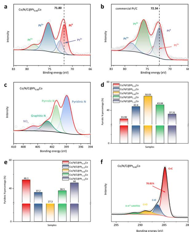
**Fig. 4** Pt 4f XPS spectra of (a) Co/N/C@Pt<sub>0.88</sub>Co and (b) commercial Pt/C. (c) N 1s XPS spectra of Co/N/C@Pt<sub>0.88</sub>Co. The content of (d) pyrrolic N and (e) pyridinic N of various Co/N/C@Pt<sub>x</sub>Co catalysts. (f) C 1s XPS spectra of Co/N/C@Pt<sub>0.88</sub>Co.
