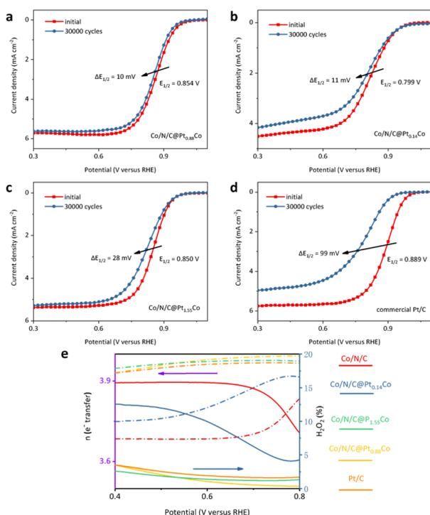
**Fig. 5** ORR polarization curves of (a) Co/N/C@Pt<sub>0.88</sub>Co, (b) Co/N/C@Pt<sub>0.14</sub>Co, (c) Co/N/C@Pt<sub>1.55</sub>Co and (d) Pt/C before and after 30 000-cycle ASTs. (e) Electron transfer number (left axis) and hydrogen peroxide production rate (right axis) of various catalysts.
