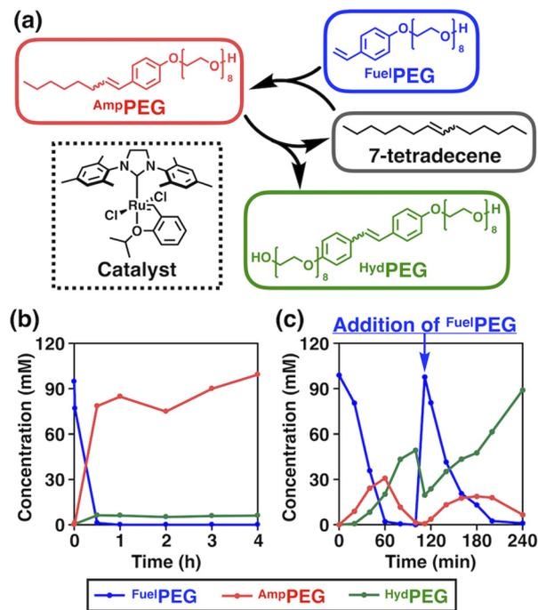
**Fig. 2** (a) Schematic illustration of the designed non-equilibrium chemical reaction system based on olefin metathesis. (b) Concentration vs. time plot of the homogeneous reaction mixture using CH<sub>2</sub>Cl<sub>2</sub> as a solvent at 25 °C (480 rpm). (c) Concentration vs. time plot of the biphasic reaction mixture using H<sub>2</sub>O as a solvent at 50 °C (480 rpm). At 100 min, FuelPEG was added as an additional “fuel”.
