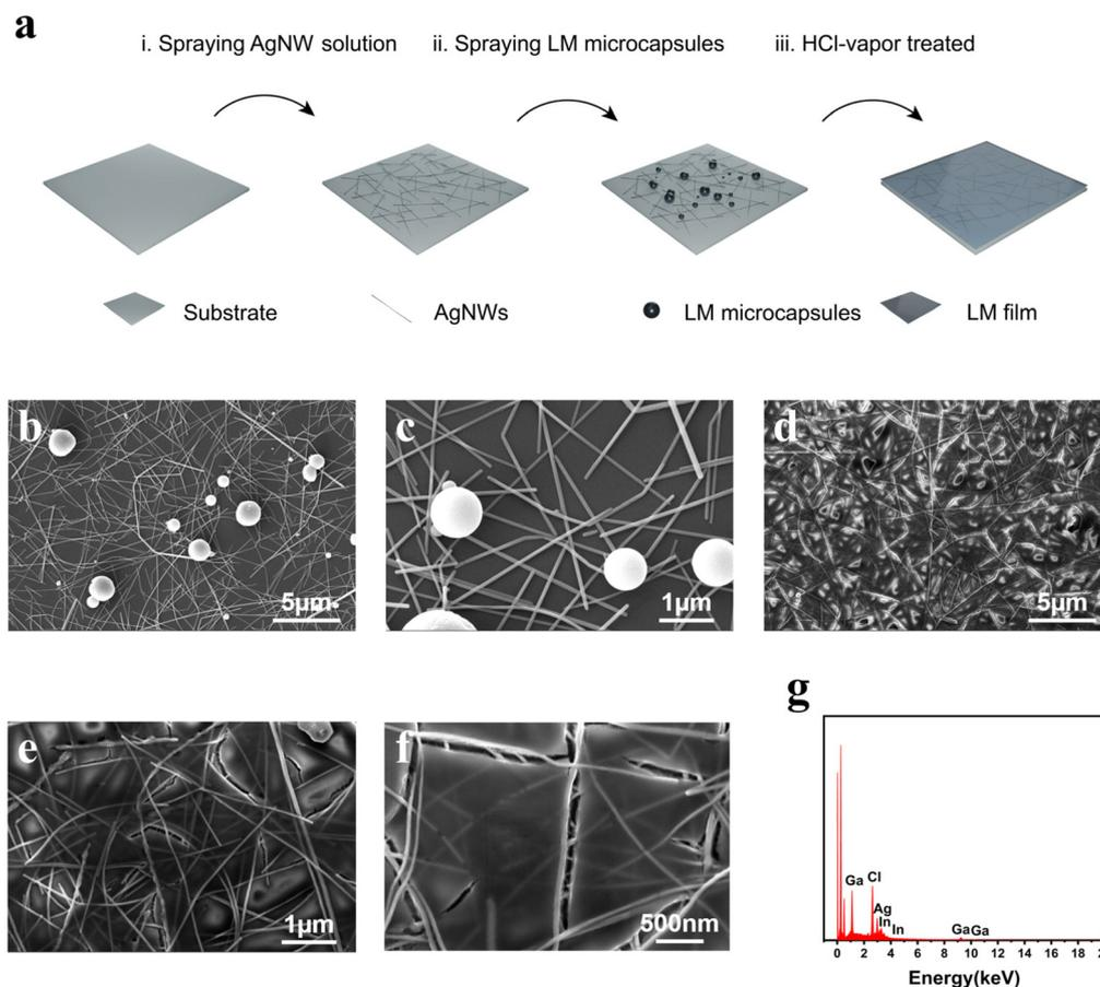
**Fig. 1** (a) Schematic illustrating the process to obtain transparent AgNW-LM conductors. (b and c) SEM images of the transparent conductor before HCl vapor treatment. (d–f) SEM images of the transparent conductor after HCl vapor treatment. (g) EDS pattern of the hybrid conductor on the substrate.
