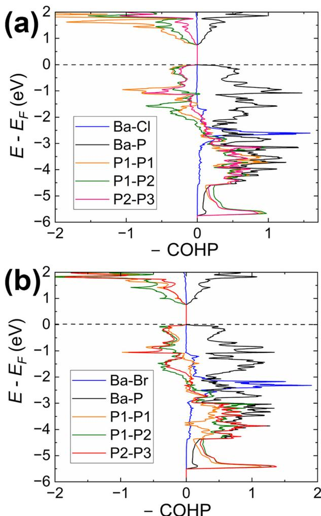
**Fig. 5** (a) COHP curves for selected averaged Ba–X and Ba–P interactions and three specific interactions (P1–P1, P1–P2, and P2–P3) within the helical  $\frac{1}{2}\text{P}$  chain in  $\text{Ba}_3\text{P}_5\text{Cl}$  (a) and  $\text{Ba}_3\text{P}_5\text{Br}$  (b) calculated for the C2/c structural model.
