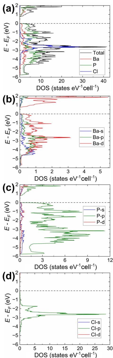
**Fig. 3** Electronic structure in  $\text{Ba}_3\text{P}_5\text{Cl}$  ( $C2/c$  structural model; Fig. S7a and Tables S1, S2<sup>†</sup>): (a) total DOS together with projected densities of states for constituting elements; (b)–(d) partial DOS calculated for the different orbitals of Ba, P, and Cl, respectively.
