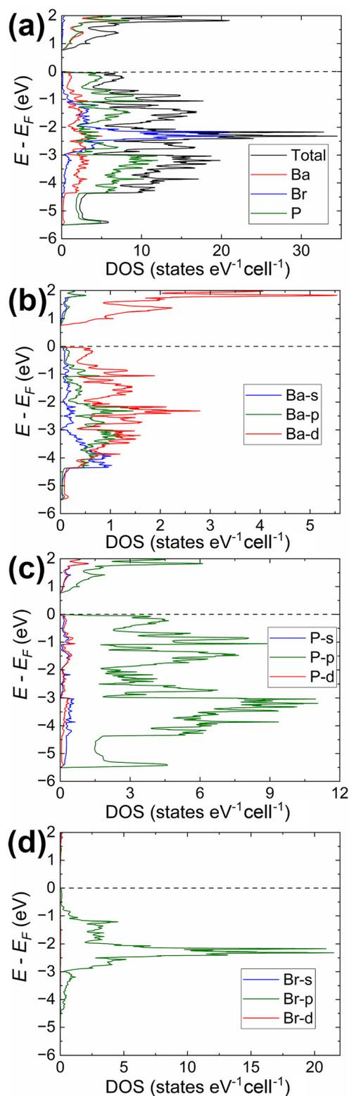
**Fig. 4** Electronic structure in  $\text{Ba}_3\text{P}_5\text{Br}$  ( $C2/c$  structural model; Fig. S7a and Tables S1, S3<sup>†</sup>): (a) total DOS together with projected densities of states for constituting elements; (b)–(d) partial DOS calculated for the different orbitals of Ba, P, and Br, respectively.
