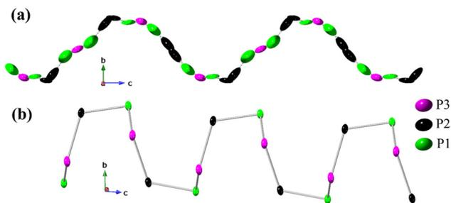
**Fig. 2** Propagation of 1D  $\frac{1}{\infty}P^{1-}$  helical chains found in (a) the crystal structures of  $Ba_3P_5X$  and (b)  $AP_2$  ( $A = Sr, Ba$ ). The P–P bonding interactions have been represented with dotted lines in  $Ba_3P_5X$ , while solid-bond has been used in the case of  $AP_2$ . Ellipsoids are plotted with a 50% probability level.
