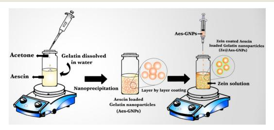
Fig. 1 Schematic representation of Ze@Aes-GNP (zein-coated aescin-loaded gelatin nanoparticles) formulation.
