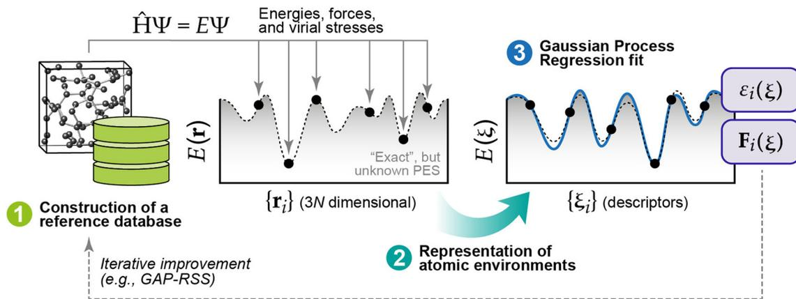
Fig. 4 Three main components required for GAPs: (1) a robust reference database of quantum-mechanical data (usually generated with DFT), (2) a representation of the atomic environments associated with each reference point, and (3) the GPR model fit. This figure has been reproduced from ref. 69 with permission from the American Chemical Society, copyright 2021.
