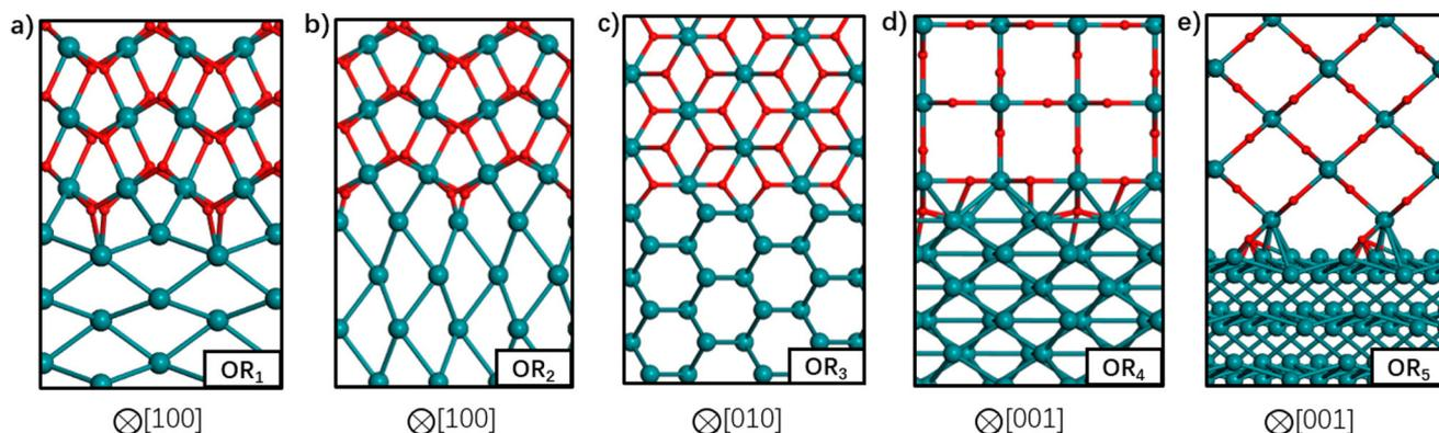
**Fig. 8** Atomic structures of the five most stable Ru–RuO<sub>2</sub> interfaces with different orientation relationships (OR) in order of increasing interfacial energy from (a) to (e). Ru atoms are depicted by the green balls and O atoms by the red balls. The crystallographic direction in RuO<sub>2</sub> bulk is indicated below each interface. This figure has been reprinted from ref. 120 with permission from the American Chemical Society, copyright 2021.
