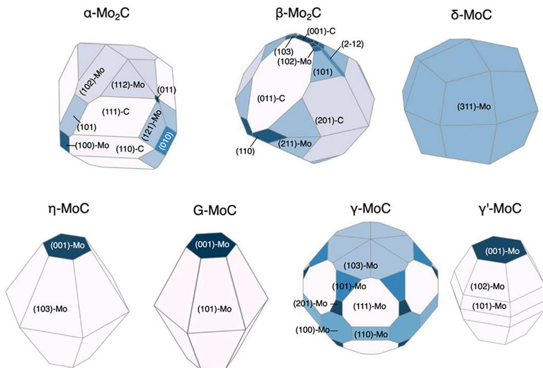
**Fig. 6** DFT-computed Wulff constructions of the equilibrium particle morphologies of different molybdenum carbide phases at  $\Delta\mu_{\text{C}} = -0.15 \text{ eV}$  using NN-identified facets. This figure has been reprinted from ref. 93 with permission from the American Chemical Society, copyright 2021.
