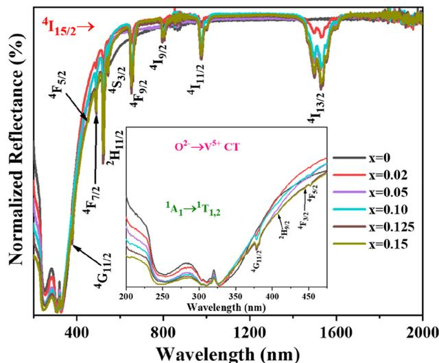
Fig. 3 UV-visible-NIR DRS of  $\text{Ba}_2\text{V}_2\text{O}_7:\text{xEr}^{3+}$  nanomaterials.
