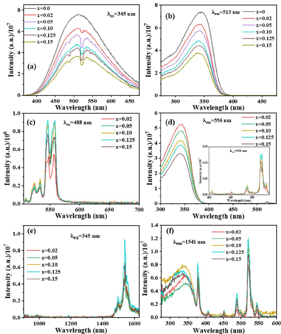
Fig. 5 Photoluminescence spectra excited at (a) 345 nm and (c) 488 nm in the visible region, (e) 345 nm in the NIR region, and excitation spectra monitored at (b) 513 nm, (d) 556 nm, and (f) 1541 nm emission of  $\text{Ba}_2\text{V}_2\text{O}_7:\text{xEr}^{3+}$  ( $x = 0-0.15$ ).
