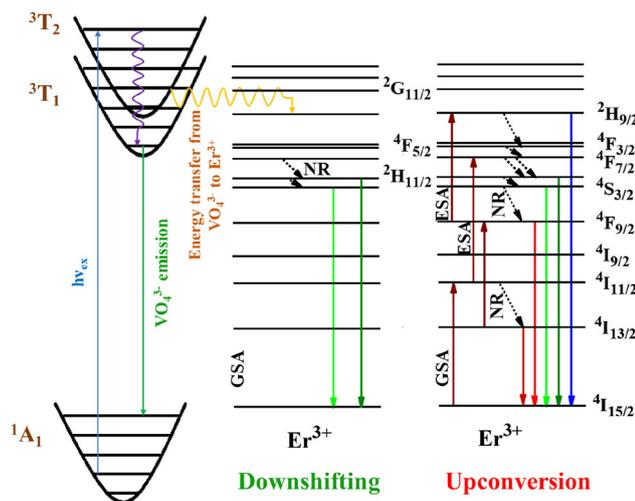
Fig. 7 Schematic of the energy levels of Er<sup>3+</sup>-doped Ba<sub>2</sub>V<sub>2</sub>O<sub>7</sub>, showing the potential transition mechanism.
