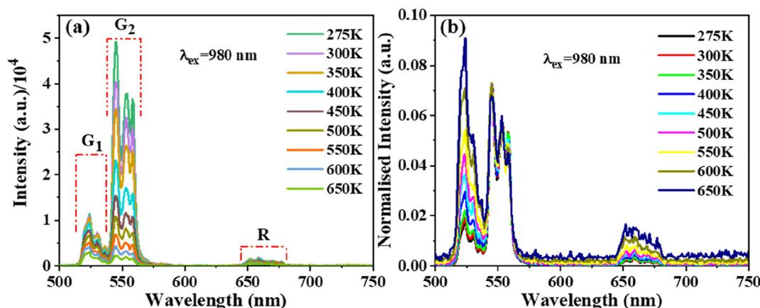
Fig. 8 Temperature-varied (a) UC PL spectra and (b) 551 nm normalized emission spectra of Ba<sub>2</sub>V<sub>2</sub>O<sub>7</sub>:0.125Er<sup>3+</sup>.
