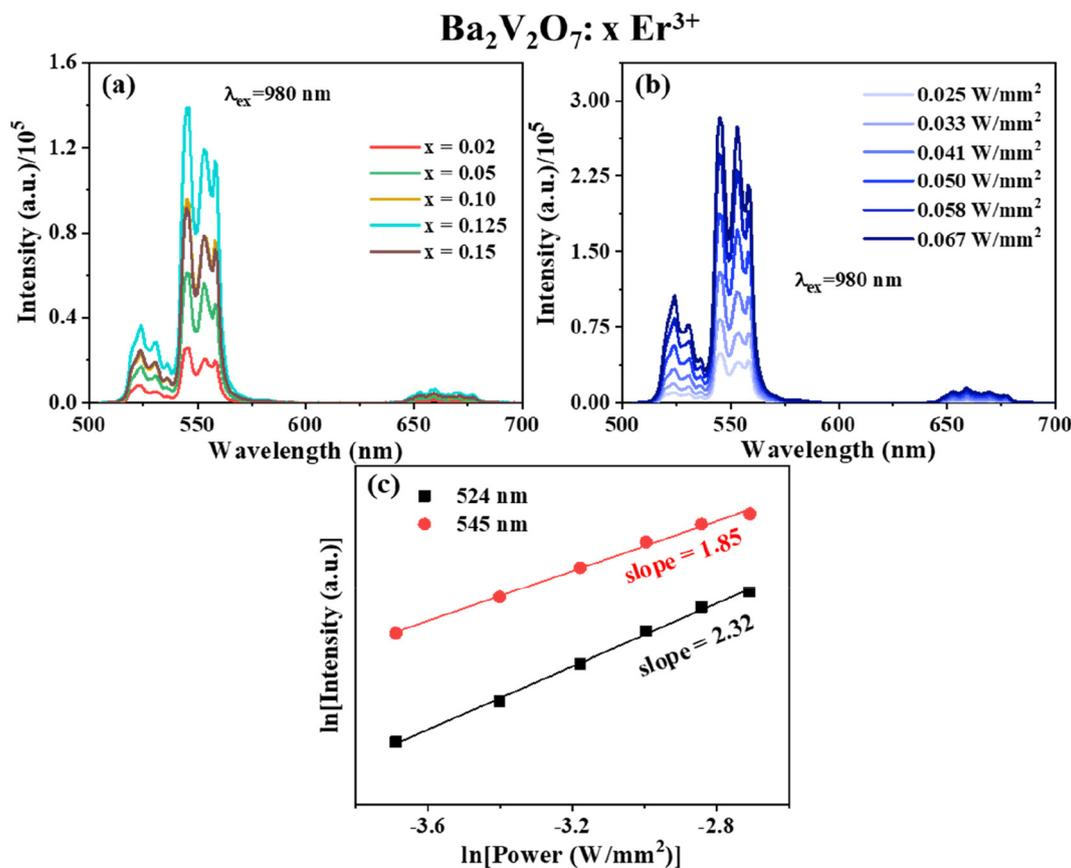
Fig. 6 (a) Upconversion luminescence of doped  $\text{Ba}_2\text{V}_2\text{O}_7:x\text{Er}^{3+}$  phosphors upon excitation with a 980 nm laser. (b) Laser power-dependent upconversion luminescence of  $\text{Ba}_2\text{V}_2\text{O}_7:0.125\text{Er}^{3+}$ . (c) Plot of  $\ln(I)$  vs.  $\ln(P)$  of  $\text{Ba}_2\text{V}_2\text{O}_7:0.125\text{Er}^{3+}$ .
