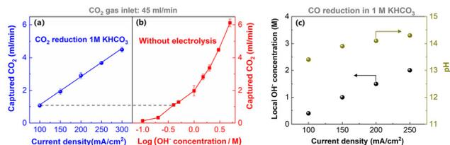
**Fig. 7** Comparison of  $\text{CO}_2$  capture rates during  $\text{CO}_2$  electrolysis at various current densities (a) and for various  $\text{KOH}$  concentration electrolytes at open-circuit potential (b). (c) The local pH in  $\text{CO}$  reduction estimated by comparing (c) with (d). This figure has been reproduced from ref. 41 with permission from Royal Society of Chemistry, copyright 2022.
