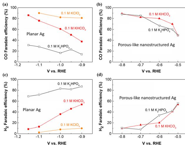
**Fig. 1** Faradaic efficiencies for CO and H<sub>2</sub> on flat Ag foil (a) (c) and porous-like nanostructured Ag (b) (d) at various potentials in 0.1 M K<sub>2</sub>HPO<sub>4</sub>, 0.1 M KHCO<sub>3</sub> or 0.1 M KClO<sub>4</sub> (all electrolytes were saturated with CO<sub>2</sub>), respectively. This figure has been reproduced from ref. 47 with permission from John Wiley and Sons, copyright 2016.
