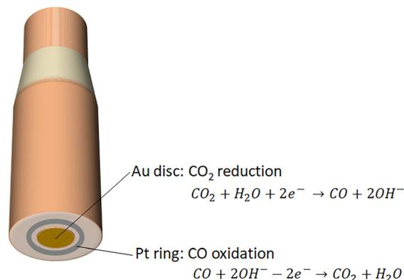
**Fig. 3** Schematic illustration of rotating ring disc electrode. Electrocatalytic CO<sub>2</sub> reduction to CO takes place on Au disc electrode, and subsequently oxidation of CO into CO<sub>2</sub> occurs on Pt ring electrode.
