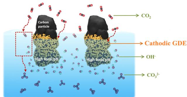
**Fig. 4** Schematic illustration of CO<sub>2</sub> capture at the cathodic GDE/catholyte interface in the form of carbonate *via* the neutralization reaction with OH<sup>-</sup> during high-rate CO<sub>2</sub> reduction. This Figure has been adapted from ref. 41 with permission from Royal Society of Chemistry, copyright 2022.
