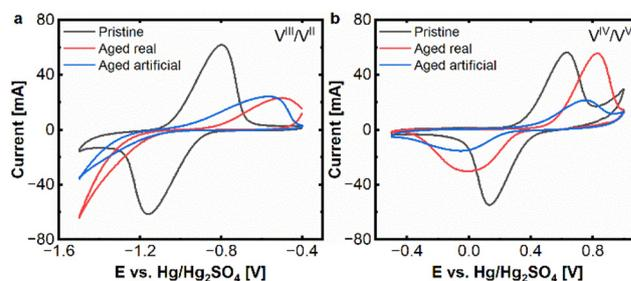
Fig. 1 CV ( $20 \text{ mV s}^{-1}$ ) real and artificial aging: (a) negative side and (b) positive side. Measured at a scan rate of  $20 \text{ mV s}^{-1}$  in an electrolyte of 15 mM  $\text{VOSO}_4 \cdot x\text{H}_2\text{O}$  dissolved in 2 M  $\text{H}_2\text{SO}_4$ .
