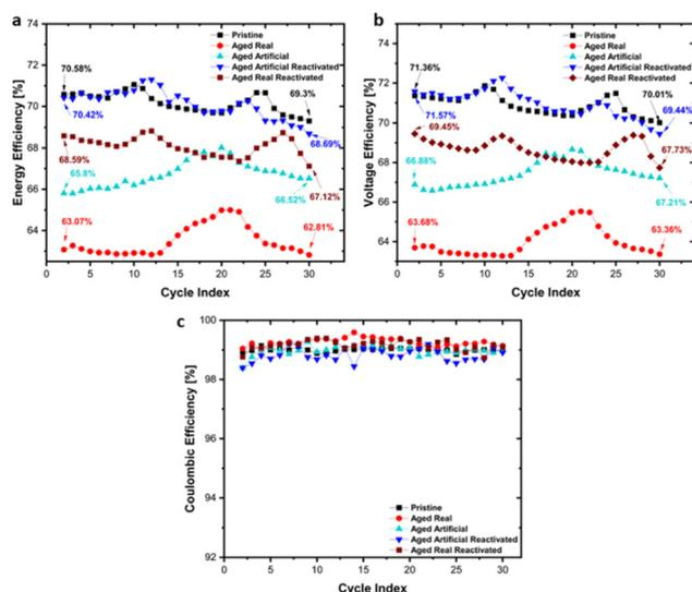
**Fig. 8** Flow cell tests on pristine carbon felt, aged real, aged artificial, and reactivated felts for 30 cycles with first and last values indicated. (a) Energy Efficiency, (b) voltage Efficiency, (c) coulombic Efficiency.
