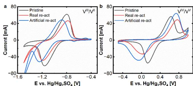
Fig. 2 CV ( $20 \text{ mV s}^{-1}$ ) thermal re-activation effect on the real and artificially aged felts: (a) negative side and (b) positive side. Measured at a scan rate of  $20 \text{ mV s}^{-1}$  in an electrolyte of  $15 \text{ mM VO}_2 \cdot x\text{H}_2\text{O}$  dissolved in  $2 \text{ M H}_2\text{SO}_4$ .
