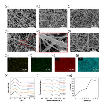
**Fig. 2** Characterization of PVDF/ZnO nanofiber films. The SEM images of PVDF/ZnO nanofibers with ZnO content of (a) 0 wt%, (b) 2 wt%, (c) 5 wt%, (d and e) 7 wt%, and (f) 10 wt%. The EDS images of PVDF/ZnO nanofibers: (g) Zn, (h) O, (i) C, and (j) F. (k) The XRD patterns of PVDF/ZnO nanofibers. (l) The FT-IR spectra of PVDF/ZnO nanofibers. (m) The calculated β-phase content of PVDF/ZnO nanofibers.
