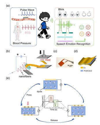
Fig. 1 Applications and design of the TCBPS. (a) Diagram of the TCBPS on monitoring different physiological signals. (b) Schematic illustration of the fabrication process for the TCBPS. (c) A photograph of the TCBPS. (d) Schematic of the multilayer structure of the TCBPS. (e) The working mechanism of the TCBPS under compression and release.
