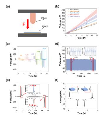
Fig. 3 Electromechanical characterization of the TCBPS. (a) Diagram of the measurement platform. (b) Voltage versus force curves for the TCBPS with different ZnO contents when the force ranges from 1 to 30 N. (c) Robust response of voltage output of the TCBPS under different magnitudes of forces. (d) Cyclic stability test of the TCBPS over 2000 cycles under 1 Hz and 5 N. (e) Response time of the TCBPS at the frequency of 1 Hz. (f) Switching polarity test under forward and reverse connections.
