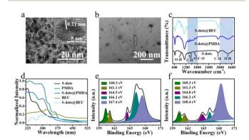
Fig. 2 Characterization of S-dots@PMDA and S-dots@BEU. TEM images of S-dots@PMDA (a) and S-dots@BEU (b). (c) FTIR spectra of S-dots, S-dots@PMDA, and S-dots@BEU, as indicated on the frame. (d) UV-visible absorption spectra of S-dots, S-dots@PMDA, S-dots@BEU, and pure molecules of PMDA and BEU, as indicated on the frame. High-resolution S 1s XPS spectra of S-dots@PMDA (e) and S-dots@BEU (f).
