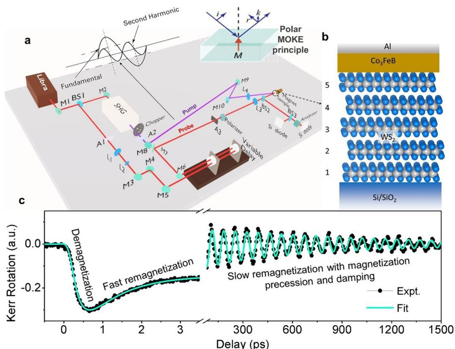
**Fig. 1** (a) TR-MOKE experimental setup. (b) Layer schematic of the  $\text{WS}_2/\text{Co}_3\text{FeB}/\text{Al}$  heterostructure. (c) Recorded data on the  $\text{WS}_2$  ( $n_{\text{ML}} = 4$ )/ $\text{Co}_3\text{FeB}$  sample at an external bias magnetic field of 1.56 kOe and a pump fluence of  $10 \text{ mJ cm}^{-2}$ . The three important temporal regimes are indicated in the graph. The black solid lines are fit to eqn (1) and (2).
