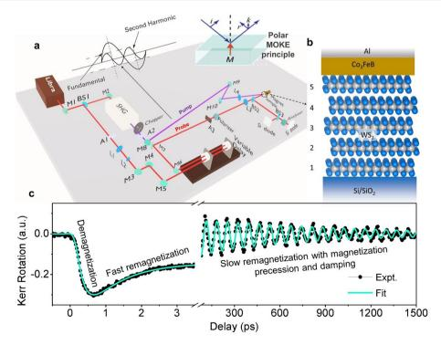
Fig. 1 (a) TR-MOKE experimental setup. (b) Layer schematic of the WS<sub>2</sub>/Co<sub>3</sub>FeB/Al heterostructure. (c) Recorded data on the WS<sub>2</sub> (n<sub>ML</sub> = 4)/Co<sub>3</sub>FeB sample at an external bias magnetic field of 1.56 kOe and a pump fluence of 10 mJ cm<sup>-2</sup>. The three important temporal regimes are indicated in the graph. The black solid lines are fit to eqn (1) and (2).
