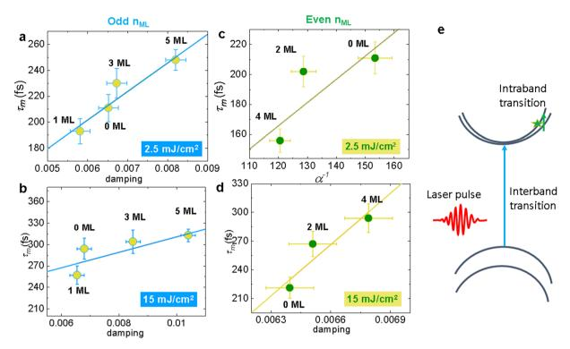
Fig. 4 Variation of  $\tau_{\rm m}$  as a function of  $\alpha$  for (a and c) lowest pump fluence and (b and d) highest pump fluence for odd  $n_{\rm ML}$  and even  $n_{\rm ML}$ , respectively. Lines in (a), (c) and (d) are fits to eqn (7), while in (b) the line is a fit to eqn (8). (e) Cartoon of laser pulse interaction resulting in inter- and intraband transitions in WS2.
