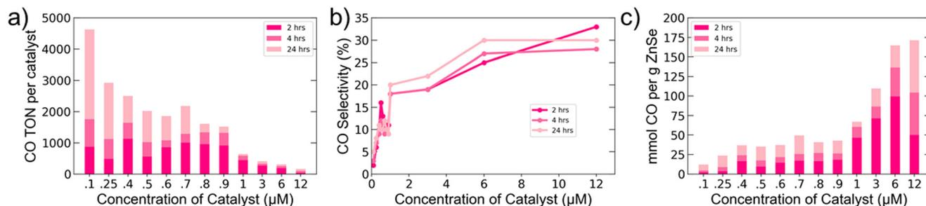
**Fig. 4** Effect of varying Co-TPP concentration on CO<sub>2</sub> reduction. (a) CO TON per catalyst, (b) CO selectivity, and (c) mmol CO produced per gram of ZnSe QDs. Photocatalysis experiments were performed on 2.0 mL aqueous solutions of 0.4 μM ZnSe QDs and 50 mM NaAsc. Samples were irradiated with 400 nm LEDs.
