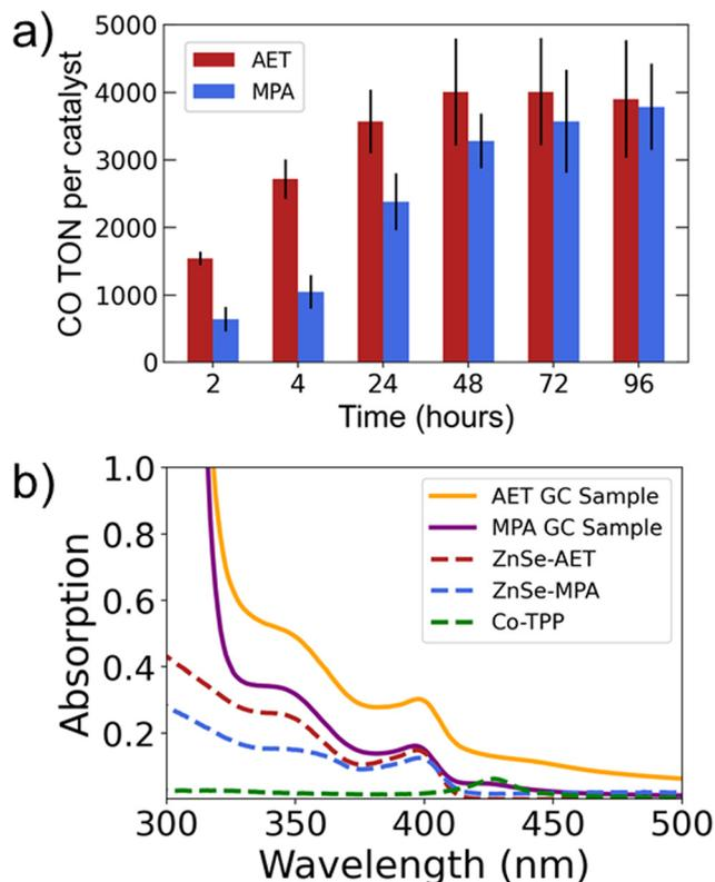
**Fig. 2** (a) Longer experiments comparing AET and MPA QDs. (b) UV-Vis spectra of reaction mixtures (GC samples) overlain with ligand-functionalized QDs and catalyst at identical concentrations alone in solution (dashed lines). Photocatalysis experiments were performed in triplicate on 2.0 mL aqueous solutions of 0.4  $\mu\text{M}$  ZnSe QDs, 0.4  $\mu\text{M}$  Co-TPP, and 100 mM NaAsc. Samples were irradiated with 400 nm LEDs.
