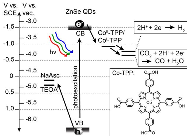
**Scheme 1** Relevant processes and energetics for photocatalytic CO<sub>2</sub> reduction using ZnSe QDs. Oxidation potentials for sacrificial hole scavengers, sodium ascorbate (NaAsc) and triethanolamine (TEOA), are shown as well as reduction potentials for the Co-TPP catalyst and relevant reactions (CO<sub>2</sub> reduction and HER).
