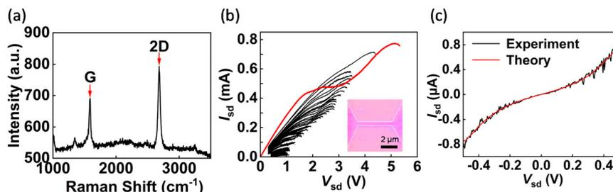
**Fig. 1** Graphene quantum dot devices fabricated by electroburning. (a) Standard Raman diagram of a single-layer graphene; compared with G peaks, the higher 2D peaks show a monolayer characteristic. (b)  $I$ - $V$  curves of the feedback electroburning process; the red line is the curve of the first cycle, and the illustration is the graphene nanoribbon diagram under a microscope. (c)  $I$ - $V$  curve after electroburning, obtained using the Simmons model to estimate the gap at 1–2 nm.
