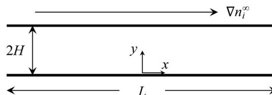
**Fig. 1** A constant concentration gradient of a binary, symmetric electrolyte  $\nabla n_i^\infty$  induces a diffusioosmotic flow in a channel that comprises two parallel plates of constant surface charge density and length  $L$  separated by distance  $2H$ . The diffusioosmotic flow is parallel to  $\nabla n_i^\infty$  along the  $x$ -direction.
