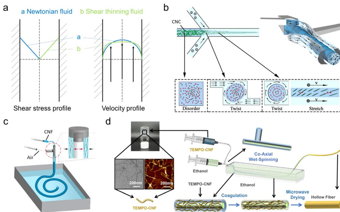
**Fig. 7** (a) Estimated shear stress profile and velocity profile within the spinning spinneret. Schematic presentation of special wet spinning spinnerets: (b) convection focusing device.<sup>70</sup> Adapted with permission from ref. 70. Copyright 2018 Elsevier. (c) Coaxial spinning device with compressed air as the inner flow.<sup>91</sup> (d) Coaxial spinning device with coagulation batch as the inner flow.<sup>125</sup> Adapted with permission from ref. 125. Copyright 2023 ACS.
