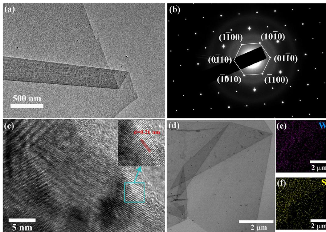
**Fig. 3** TEM images of transferred  $WS_2$  flakes. (a) Freestanding monolayer  $WS_2$  flake, folded during the transfer process. (b) Hexagonal diffraction (SAED) pattern on monolayer  $WS_2$ . (c) HRTEM image with lattice planes; the inset shows an interplanar spacing of 0.26 nm. (d) EDS elemental mapping of  $WS_2$  flakes. (e) and (f) Elemental mapping of tungsten and sulfur, respectively.
