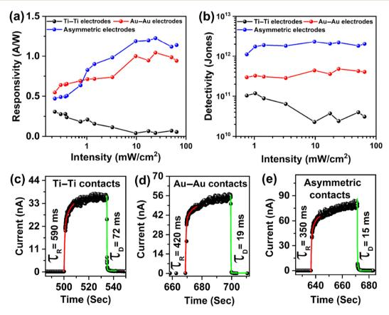
Fig. 8 (a) A comparison of the responsitivity of bilayer WS2 PDs for different metal electrode combinations. (b) A comparison of the detectivity of bilayer WS<sub>2</sub> PDs based on different metal electrode combinations. (c-e) Temporal photocurrent responses and time constants of symmetric Ti-Ti and Au-Au and asymmetric Ti-Au contact based bilayer WS<sub>2</sub> PDs.
