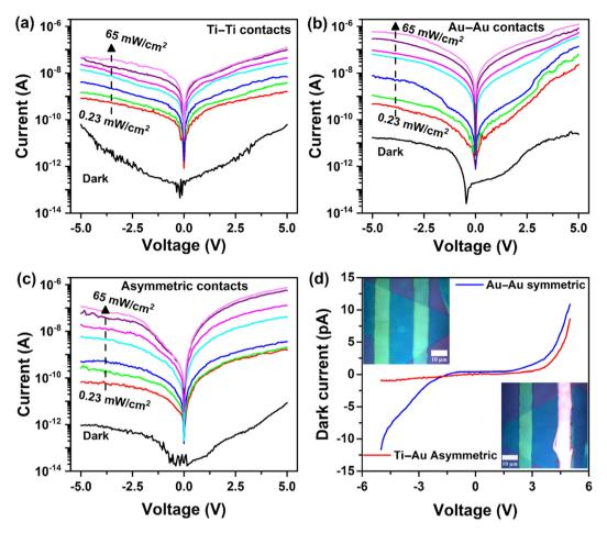
Fig. 6 Dark and photo I-V characteristics of the WS<sub>2</sub> PD. (a-c) I-V characteristics of WS<sub>2</sub>-based PDs under 405 nm laser illumination at different intensities corresponding to symmetric Ti-Ti, symmetric Au-Au and asymmetric (Ti-Au) contact-based systems, respectively. (d) A comparison of the dark currents for symmetric Au-Au contacts and asymmetric Ti-Au contacts; the inset shows optical images of PDs with symmetric (top left) and asymmetric (bottom right) contacts.
