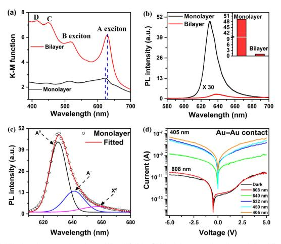
Fig. 4 (a) UV-visible absorption spectra of monolayer and bilayer  $WS_2$  flakes. (b) PL emission spectra of monolayer and bilayer  $WS_2$  under 532 nm laser excitation. The inset shows the bar diagram of the relative PL intensity for monolayer and bilayer  $WS_2$ . (c) Deconvoluted PL emission spectrum for monolayer  $WS_2$ . (d) Excitation wavelength dependent photo I-V characteristics of the  $WS_2$  PD for symmetric Au contacts.
