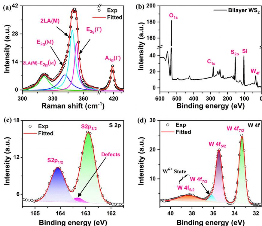
**Fig. 2** (a) Deconvoluted Raman spectra of bilayer WS<sub>2</sub> under 532 nm laser excitation. (b) XPS survey spectra of CVD-grown bilayer WS<sub>2</sub>. (c) The high-resolution core binding energy spectrum of sulfur (S). (d) The high-resolution core binding energy spectrum of tungsten (W).
