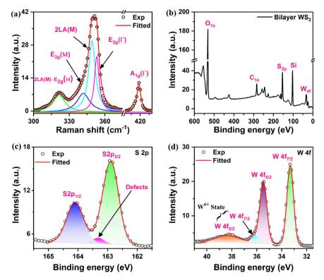
Fig. 2 (a) Deconvoluted Raman spectra of bilayer  $WS_2$  under 532 nm laser excitation. (b) XPS survey spectra of CVD-grown bilayer  $WS_2$ . (c) The high-resolution core binding energy spectrum of sulfur (S). (d) The high-resolution core binding energy spectrum of tungsten (W).
