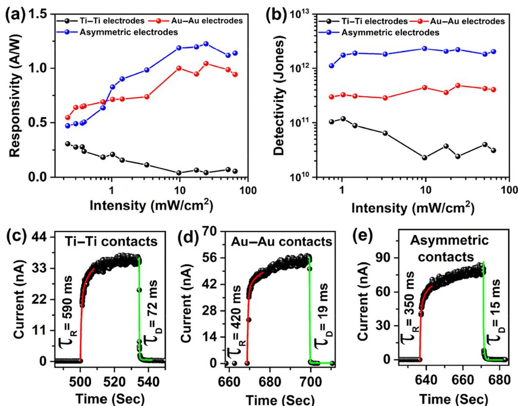
**Fig. 8** (a) A comparison of the responsivity of bilayer WS<sub>2</sub> PDs for different metal electrode combinations. (b) A comparison of the detectivity of bilayer WS<sub>2</sub> PDs based on different metal electrode combinations. (c–e) Temporal photocurrent responses and time constants of symmetric Ti–Ti and Au–Au and asymmetric Ti–Au contact based bilayer WS<sub>2</sub> PDs.
