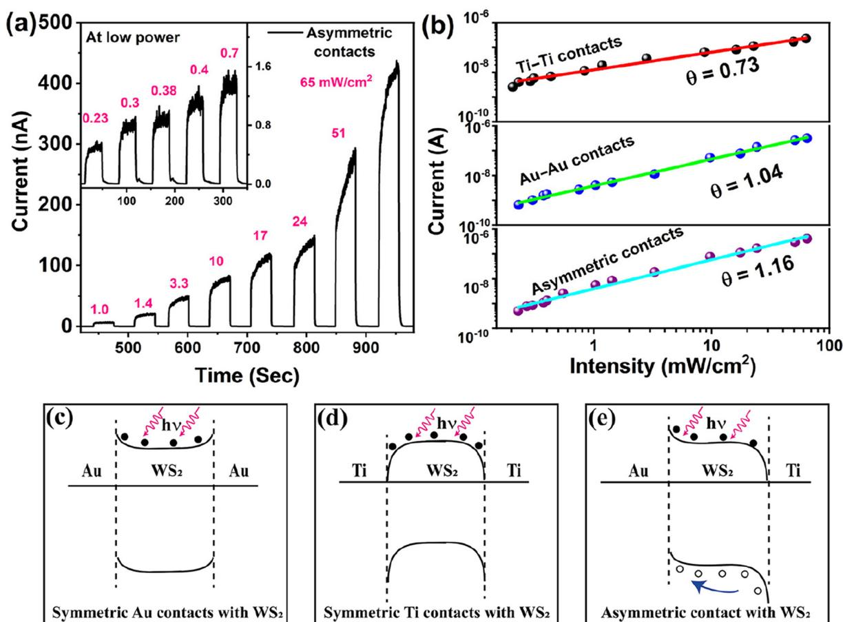
Fig. 7 (a) Photocurrent response under pulsed 405 nm laser illumination at different intensities for  $\text{WS}_2$ -based PDs with asymmetric Ti–Au contacts. (b) The photoresponse calibration curve as a function of illumination intensity for three different configurations of the PDs. Band diagrams of the  $\text{WS}_2$  based PDs under illumination conditions at zero bias for (c) symmetric Au–Au contacts, (d) symmetric Ti–Ti contacts, and (e) asymmetric Au–Ti contacts with  $\text{WS}_2$ .
