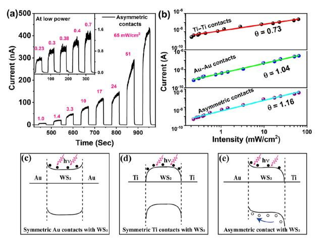
Fig. 7 (a) Photocurrent response under pulsed 405 nm laser illumination at different intensities for WS<sub>2</sub>-based PDs with asymmetric Ti–Au contacts. (b) The photoresponse calibration curve as a function of illumination intensity for three different configurations of the PDs. Band diagrams of the WS<sub>2</sub> based PDs under illumination conditions at zero bias for (c) symmetric Au–Au contacts, (d) symmetric Ti–Ti contacts, and (e) asymmetric Au–Ti contacts with WS<sub>2</sub>.
