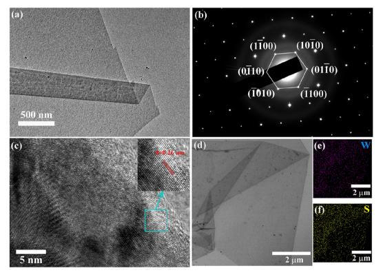
Fig. 3 TEM images of transferred WS<sub>2</sub> flakes. (a) Freestanding monolayer WS<sub>2</sub> flake, folded during the transfer process. (b) Hexagonal diffraction (SAED) pattern on monolayer WS<sub>2</sub>. (c) HRTEM image with lattice planes; the inset shows an interplanar spacing of 0.26 nm. (d) EDS elemental mapping of WS<sub>2</sub> flakes. (e) and (f) Elemental mapping of tungsten and sulfur, respectively.
