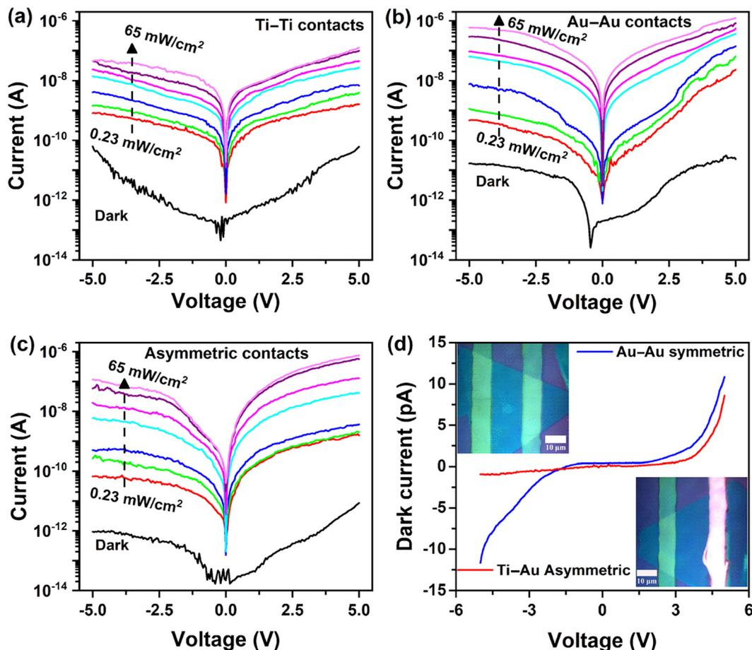
**Fig. 6** Dark and photo  $I$ - $V$  characteristics of the  $WS_2$  PD. (a–c)  $I$ - $V$  characteristics of  $WS_2$ -based PDs under 405 nm laser illumination at different intensities corresponding to symmetric Ti–Ti, symmetric Au–Au and asymmetric (Ti–Au) contact-based systems, respectively. (d) A comparison of the dark currents for symmetric Au–Au contacts and asymmetric Ti–Au contacts; the inset shows optical images of PDs with symmetric (top left) and asymmetric (bottom right) contacts.
