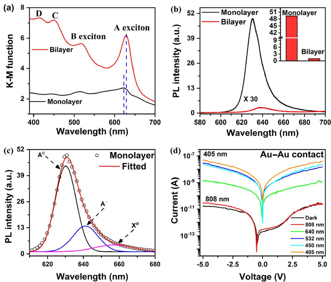
Fig. 4 (a) UV-visible absorption spectra of monolayer and bilayer WS<sub>2</sub> flakes. (b) PL emission spectra of monolayer and bilayer WS<sub>2</sub> under 532 nm laser excitation. The inset shows the bar diagram of the relative PL intensity for monolayer and bilayer WS<sub>2</sub>. (c) Deconvoluted PL emission spectrum for monolayer WS<sub>2</sub>. (d) Excitation wavelength dependent photo *I*–*V* characteristics of the WS<sub>2</sub> PD for symmetric Au contacts.
