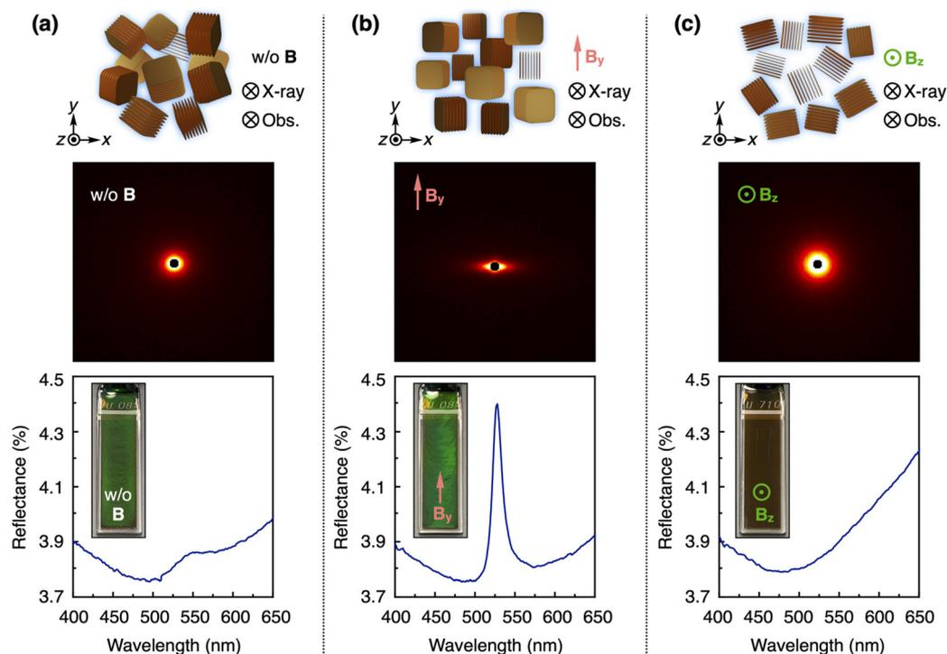
**Fig. 2** (a–c) Schematic illustrations of the orientation of GO nanosheets and 2D SAXS profiles of the gel samples of GO nanosheets ([GO] = 0.1 wt%) obtained by photo-polymerization of acrylic monomers and crosslinkers (upper) and reflection spectra (lower) with optical images (inset) of the photonic crystals of GO nanosheets ([GO] = 0.3 wt%) prepared without magnetic application (a) and with a 12 T magnetic application along the y-axis (b) and z-axis (c).
