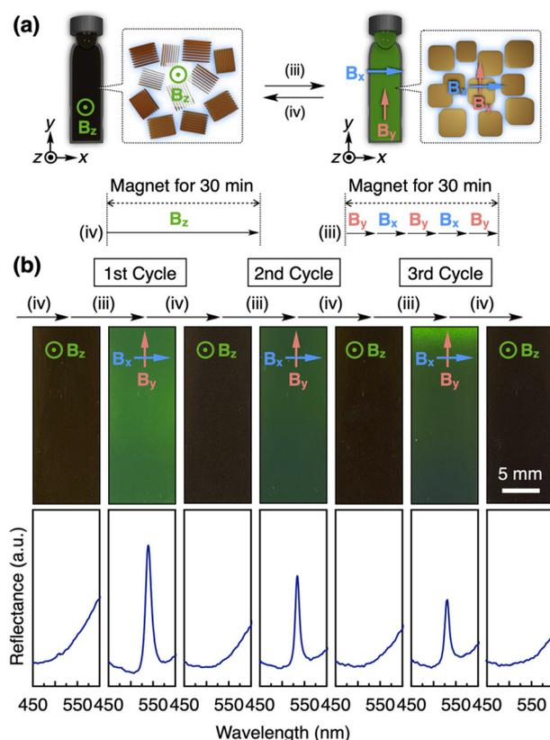
**Fig. 6** (a) Magnetic application processes (iii–iv) and their schematic illustrations for color switching. (b) Optical images (upper) and the corresponding reflection spectra (lower) of a photonic crystal of GO nanosheets ([GO] = 0.3 wt%) after repeating processes (iii) and (iv).
