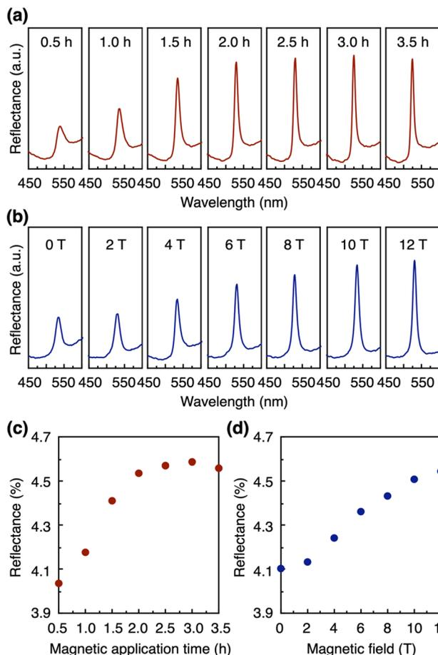
**Fig. 4** (a–d) Reflection spectra (a and b) and plots of peak intensity in the spectra (c and d) as a function of the application time of a 12 T magnetic field at 50 °C (a and c) and the magnetic strength with an application time of 3 h (b and d) using a photonic crystal of GO nanosheets ([GO] = 0.3 wt%) with the magnetic treatment along the *y*-axis.
