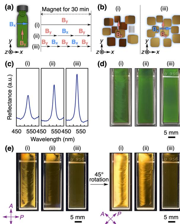
**Fig. 5** (a) Magnetic application processes (i–iii) for improving the quality of a structural color. A 12 T magnetic field was alternately applied along the *y*- and *x*-axis directions with a total magnetic application time of 30 min at 50 °C. (b) Schematic illustrations of the orientation of GO nanosheets after processes (i) and (iii). (c) Reflection spectra, (d) optical images, and (e) polarized optical images of a photonic crystal of GO nanosheets ([GO] = 0.3 wt%) after processes (i–iii).
