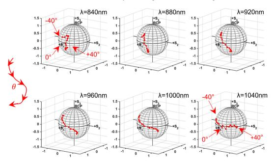
Fig. 6 Evolution of the output polarization vector on the Poincaré sphere, tuned with the incidence angles from -40° to +40°, at different excitation wavelengths; the excitation light is always p-polarized.
