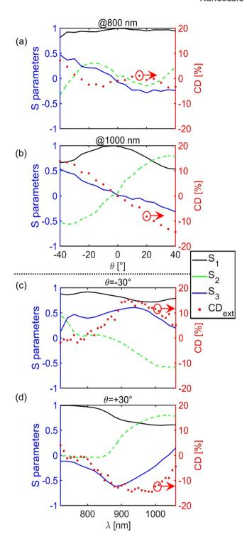
Fig. 4 (a) S parameters of the output light, when the metasurface is excited with p-polarized light, and its comparison to the extinction CD for incidence angle rotation at (a) 800 nm and (b) 1000 nm; (c and d) tuning the excitation wavelength for (c)  $\theta = -30^{\circ}$  and (d)  $\theta = +30^{\circ}$ .
