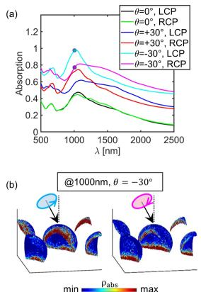
Fig. 3 (a) Calculated absorption shows extrinsic chiral behaviour resonating at around 1000 nm; for the sake of clarity,  $\theta = +30^{\circ}$  and  $\theta = -30^{\circ}$  lines are vertically shifted by 0.2 and 0.4, respectively. (b) Excitation at 1000 nm resonance leads to a large difference in the absorption density between LCP and RCP for  $\theta = -30^{\circ}$ .
