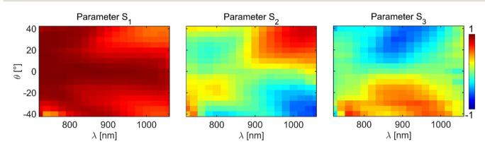
Fig. 5 Full characterization of the S parameters of the transmitted light, dependent on the excitation wavelength  $\lambda$  and incidence angle  $\theta$ .
