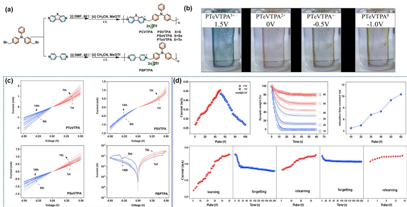
**Fig. 7** (a) Synthesis of PCVTTPA (PSVTTPA, PSeVTTPA, PTeVTTPA) and PBPTTPA. (b) Electrochromic photographs of the PTeVTTPA thin film coated onto the ITO substrate. (c) *I*–*V* characteristics of the Al/polymer/ITO devices. (d) Synaptic function simulation in human brain memory behavior, including repetitive learning forgetting (STP/STD).<sup>97</sup> Reprinted with permission from ref. 97 © 2021 Open Access.
