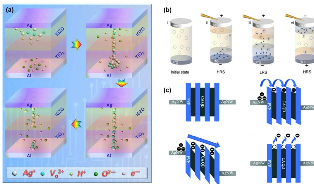
**Fig. 4** (a) Schematic illustration of the formation of conductive filaments.<sup>96</sup> (b) Model of the resistive switching mechanism.<sup>118</sup> (c) Schematic band diagrams to explain the resistive switching model.<sup>122</sup> Reprinted with permission from ref. 96, © 2021 American Chemical Society; ref. 118, © 2022 Science China Press and Springer; ref. 122, © 2018 Royal Society of Chemistry.
