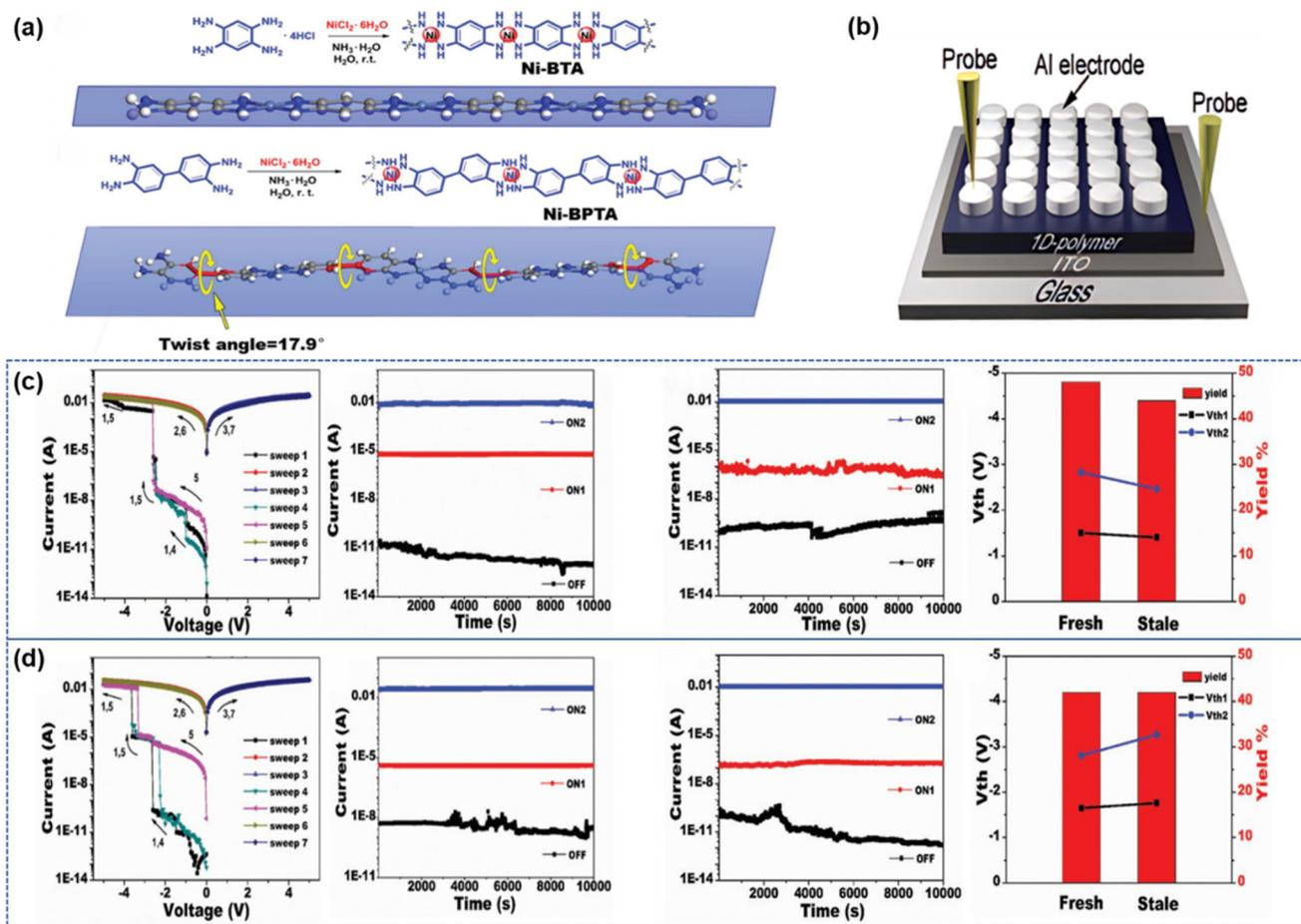
Fig. 8 (a) Synthetic routes and geometry of Ni-BTA and Ni-BPTA. (b) Typical sandwiched structure of memory devices. (c and d) Characteristic  $I$ - $V$  curves, stability, threshold voltage and ternary device yield of (c) Ni-BTA and (d) Ni-BPTA.<sup>93</sup> Reprinted with permission from ref. 93, © 2017 Wiley.
