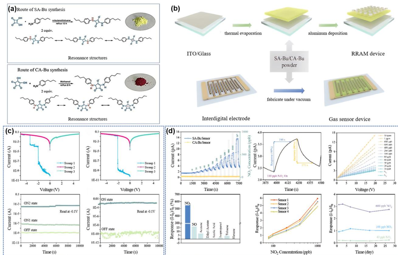
**Fig. 6** (a) Synthetic routes of SA-Bu, CA-Bu and their zwitterionic resonance structures. (b) Schematic diagram of fabricating RRAM and gas sensor devices. (c) Typical tri-state  $I-V$  and stability test characteristics of SA-Bu/CA-Bu based memory devices. (d) Transient response of SA-Bu and CA-Bu sensors with an increase in  $\text{NO}_2$  concentration.<sup>128</sup> Reprinted with permission from ref. 128, © 2021 Elsevier.
