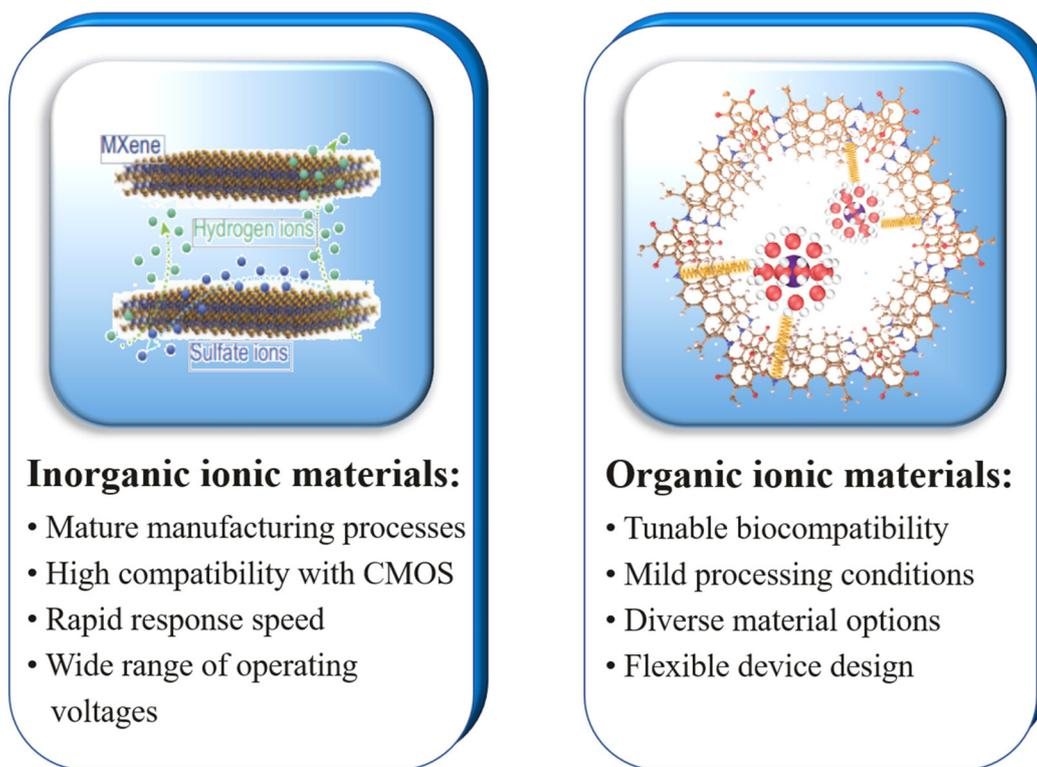
**Fig. 2** The performance comparison between inorganic ionic memristive materials and organic ionic memristive materials.<sup>71,72</sup> Reprinted with permission from ref. 71, © 2022 Oxford University Press; ref. 72, © 2021 Wiley.
