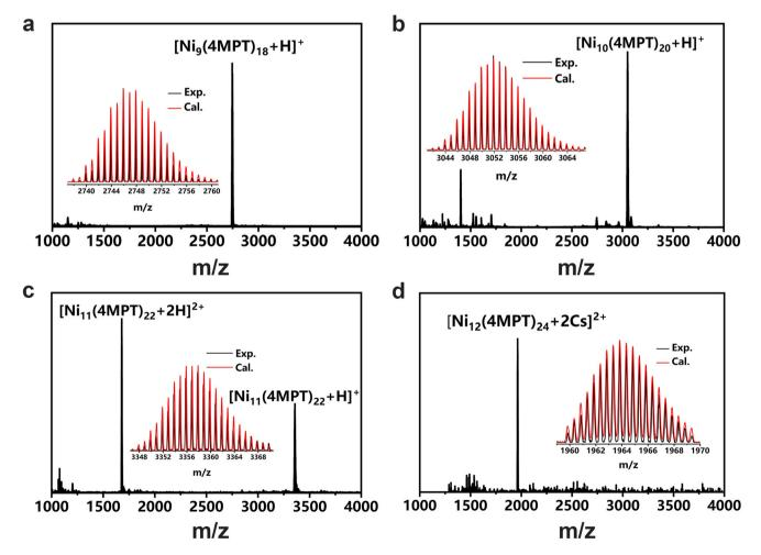
Fig. 2 ESI-MS of the  $Ni_n(4MPT)_{2n}$  clusters. (a)  $Ni_9(4MPT)_{18}$ . (b)  $Ni_{10}(4MPT)_{20}$ . (c)  $Ni_{11}(4MPT)_{22}$ . (d)  $Ni_{12}(4MPT)_{24}$ . Inset: the measured (black) and simulated (red) isotopic distribution patterns of the corresponding molecular ion peaks.
