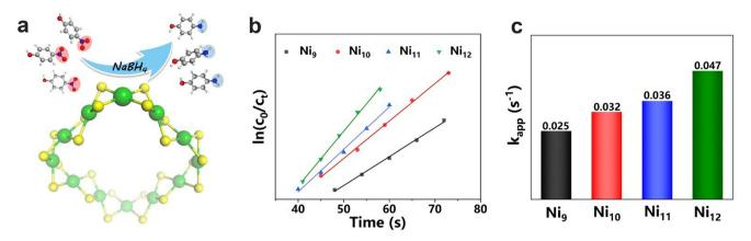
Fig. 5 Catalytic properties of the  $Ni_n(4MPT)_{2n}$  (n = 9-12) clusters in the reduction reaction of p-nitrophenol. (a) A schematic diagram for p-nitrophenol reduction. (b) The corresponding reaction kinetics of the reactions. (c) Reaction rate constant ( $k_{app}$ ) of the reduction reactions catalyzed by the clusters. Color codes: yellow sphere, S; green sphere, Ni. red sphere, O; blue sphere, N; gray sphere, C; white sphere, H.
