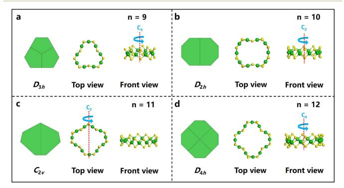
Fig. 1 Structure analysis of the  $Ni_n(4MPT)_{2n}$  clusters. (a)  $Ni_9(4MPT)_{18}$ . (b)  $Ni_{10}(4MPT)_{20}$ . (c)  $Ni_{11}(4MPT)_{22}$ . (d)  $Ni_{12}(4MPT)_{24}$ . Color codes: yellow sphere, S; green sphere, Ni. All C and H atoms are omitted for clarity.
