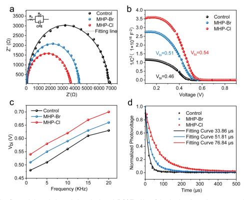
Fig. 4 (a) Nyquist plots (inserted picture is the equivalent circuit model). (b) The Mott–Schottky plot of capacitance *versus* voltage measured under 1 kHz. (c) The extracted  $V_{\text{bi}}$  values of the CQD devices under different frequencies. (d) Photovoltage decay spectra of the CQD solar cells.
