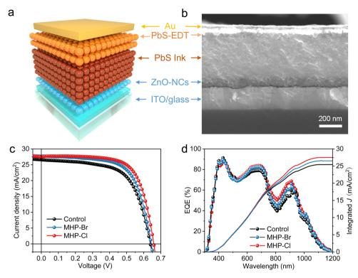
Fig. 3 (a) Schematic illustration of the CQD photovoltaic device. (b) Cross-section SEM image of the PbS CQD photovoltaic device used in this study. (c) J-V curves of CQD solar cells obtained under an AM 1.5G solar simulator. (d) EQE curves and integrated JSC of the best devices.
