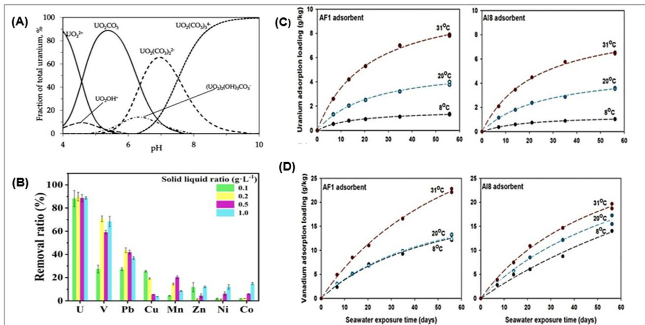
Fig. 8 (A) Speciation of uranium.<sup>20,41,162,163</sup> (B) The uranium adsorption selectivity of P-HBP-AO.<sup>45</sup> (C) Uranium time series measurements; and (D) loadings of vanadium adsorbed at 8, 20, and 31 degrees Celsius using the AF1 and A18 adsorbents. A one-site ligand saturation model was used to create the fitted lines that were drawn through the data points.<sup>75</sup>
