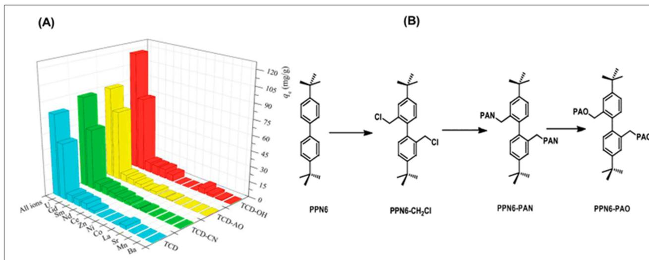
**Fig. 6** (A) The effectiveness of TCD COF and its derivatives in the aqueous solution for the selective recovery of uranium over 11 other competing ions. The experiment was run for three hours at 25 °C and pH 4.5. At first, each metal was introduced at a concentration of 0.5 mmol L<sup>-1</sup>.<sup>123</sup> (B) Method for generating amidoxime-functionalized POP synthetically (PPN-6-PAO).<sup>138</sup>
