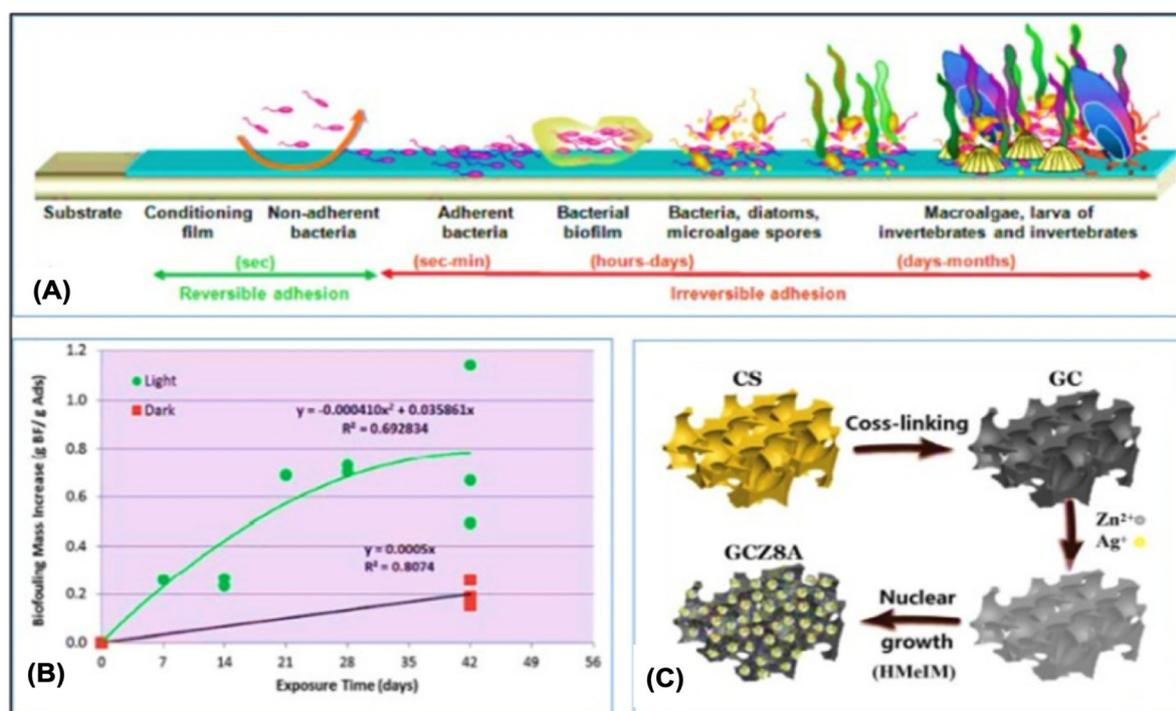
Fig. 10 (A) Marine fouling development methods.<sup>187</sup> (B) Elevation in the dry mass of the biofouling material with time in both light and dark streams. Biofouling mass is a representation of the biofouling material accumulated during 42 days (g)<sup>188</sup> per adsorbent mass (g). (C) Illustrative GCZ8A composites synthesis schematic proposed.<sup>56</sup>
