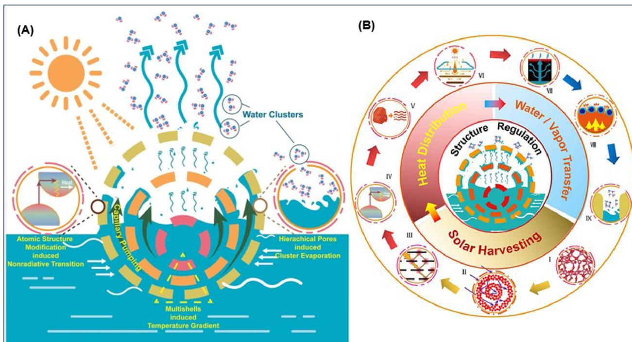
Fig. 9 (A) Illustration of the very efficient solar-to-vapor production method using amorphous Ta<sub>2</sub>O<sub>5</sub>/C HoMS of amorphous Ta<sub>2</sub>O<sub>5</sub>/C HoMS for highly efficient solar-to-vapor production.<sup>176</sup> (B) Regulation of the solar vapor generating structure affects each of the subsequent processes in the process, such as heat distribution, water/vapor transfer, and solar harvesting.<sup>194</sup>
