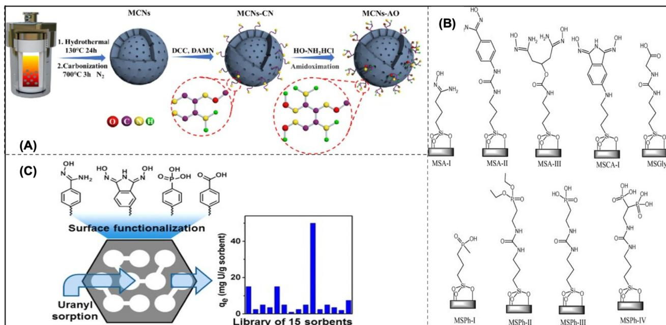
Fig. 7 (A) The MCNs-AO preparation scheme.<sup>137</sup> (B) Mesoporous silica sorbents with organo functionalization for removing U from both artificial seawater and water.<sup>139</sup> (C) Adsorbents made of functionalized mesoporous carbon.<sup>140</sup>
