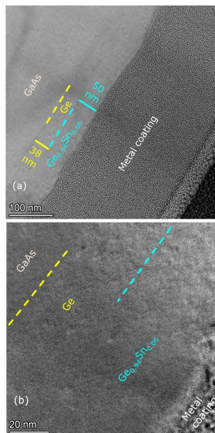
**Fig. 5** Cross-sectional TEM micrographs of sample A2: (a)  $\text{Ge}_{0.94}\text{Sn}_{0.06}/\text{Ge}/(100)/2^\circ$  GaAs heterostructure representing good quality growth of 50 nm  $\text{Ge}_{0.94}\text{Sn}_{0.06}$  grown over 38 nm thick Ge layer grown on GaAs, where broken lines demarcate similar structure factored Ge and  $\text{Ge}_{0.94}\text{Sn}_{0.06}$  epilayers, and (b) HR-TEM micrograph affirms the fine quality of the GeSn/Ge heterostructure system.
