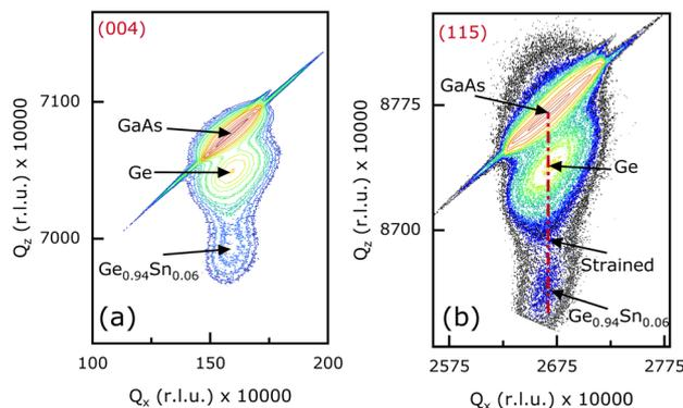
**Fig. 3** Reciprocal space maps (RSMs) taken along the (a) (004) and (b) (115) orientations, that shows  $\sim 0.81\%$  compressive strain in the 100 nm thick  $\text{Ge}_{0.94}\text{Sn}_{0.06}$  epitaxial layer (sample B1) grown on 27 nm Ge layer/(100)/6° GaAs substrate.
