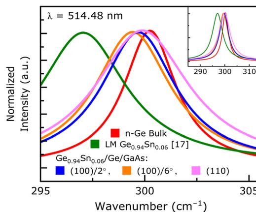
**Fig. 6** Raman spectra recorded from epitaxial  $\text{Ge}_{0.94}\text{Sn}_{0.06}$  layers of samples A1, B2 and C (compressively strained heterostructures), selectively chosen with different orientations alongside a lattice matched  $\text{Ge}_{0.94}\text{Sn}_{0.06}$  epilayer.<sup>17</sup> Positive Raman wavenumber shifts (representing compressively strained states) are observed on all three samples A1: (100)/2°, B2: (100)/6°, and C: (110).
