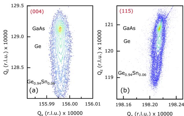
**Fig. 4** Reciprocal space maps (RSMs) taken along the (a) (004) and (b) (115) orientations show 100 nm thick  $\text{Ge}_{0.94}\text{Sn}_{0.06}$  epitaxial layer (sample C) grown on 27 nm Ge layer/(110) GaAs substrate.
