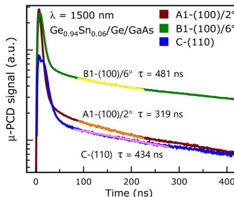
**Fig. 8**  $\mu$ -PCD signal *versus* time acquired at 300 K with 1500 nm excitation wavelength from samples A1 [(100)/2°  $\text{Ge}_{0.94}\text{Sn}_{0.06}$ ], B1 [(100)/6°  $\text{Ge}_{0.94}\text{Sn}_{0.06}$ ] and C [(110)  $\text{Ge}_{0.94}\text{Sn}_{0.06}$ ]. The corresponding minority carrier lifetimes of  $\sim 319$  ns,  $\sim 481$  ns and  $\sim 434$  ns were obtained by fitting to exponential decay after the initial surface recombination induced decay.
