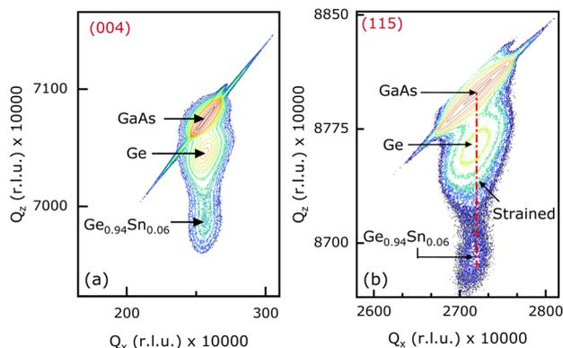
Fig. 2 Reciprocal space maps (RSMs) taken along the (a) (004) and (b) (115) orientations, that shows  $\sim 0.81\%$  compressive strain in the 100 nm thick  $\text{Ge}_{0.94}\text{Sn}_{0.06}$  epitaxial layer (sample A1) grown on 27 nm Ge/(100)/ $2^\circ$  GaAs substrate.
