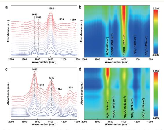
Fig. 3 In situ ATR-SEIRAS spectra of (a and b) Bi NPs@PG and (c and d) Bi SPs@PG in CO2-saturated 0.1 M KHCO3 solution from 0.1 V to -1.9 V vs. RHE
