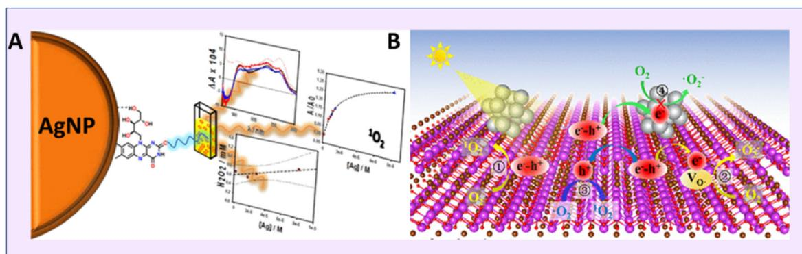
**Fig. 15** Schematic representation of singlet oxygen generation from silver nanoparticles. (A) Pectin-stabilized Ag NP. Reproduced with permission.<sup>76</sup> Copyright 2016, American Chemical Society. (B) Defect-free Au NP from FL-BiOBr-NS for enhanced SOG. Reproduced with permission.<sup>77</sup> Copyright 2022, American Chemical Society.
