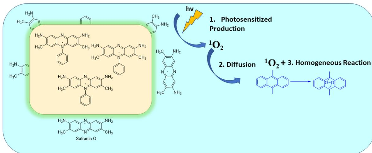
Fig. 8 Schematic representation of the photosensitized oxidation of DMA using SF/SiO<sub>2</sub> composite. This image was taken from ref. 40.
