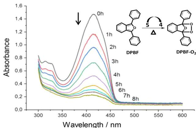
Fig. 10 <sup>1</sup>O<sub>2</sub> produced by thermolyzing M-EPO reacts with DPBF. Reproduced with permission.<sup>46</sup> Copyright 2020, American Chemical Society.
