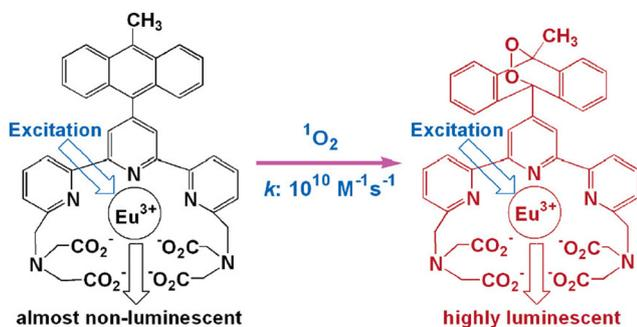
Fig. 12 Reaction of MTTA–Eu<sup>3+</sup> with <sup>1</sup>O<sub>2</sub>. Reproduced with permission.<sup>51</sup> Copyright 2006, American Chemical Society.
