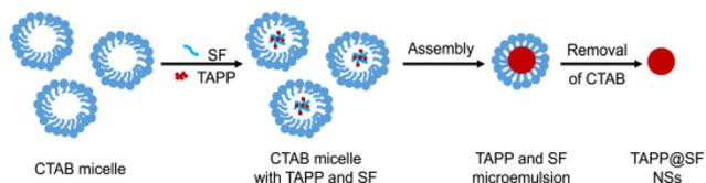
**Fig. 22** Schematic representation of preparing TAPP NSs. Reproduced with permission.<sup>144</sup> Copyright 2023, Elsevier.
