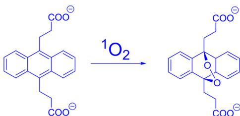
**Fig. 7** ADPA's reactivity in the presence of <sup>1</sup>O<sub>2</sub>. Reproduced with permission.<sup>36</sup> Copyright 2016, Elsevier.
