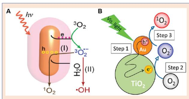
**Fig. 14** Schematic representation of singlet oxygen generation from gold nanoparticles. (A) Au nanorod. Reproduced with permission.<sup>73</sup> Copyright 2014, Royal Society of Chemistry. (B) Au NP-TiO<sub>2</sub> core-shell architecture for enhanced SOG. Reproduced with permission.<sup>71</sup> Copyright 2014, American Chemical Society.
