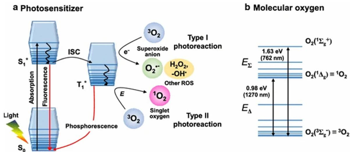
Fig. 2 (a) Jablonski diagram showing the formation of singlet oxygen via the transfer of triplet energy from a photosensitizer; (b) relative configuration of molecular oxygen's electronic states.<sup>15</sup>
