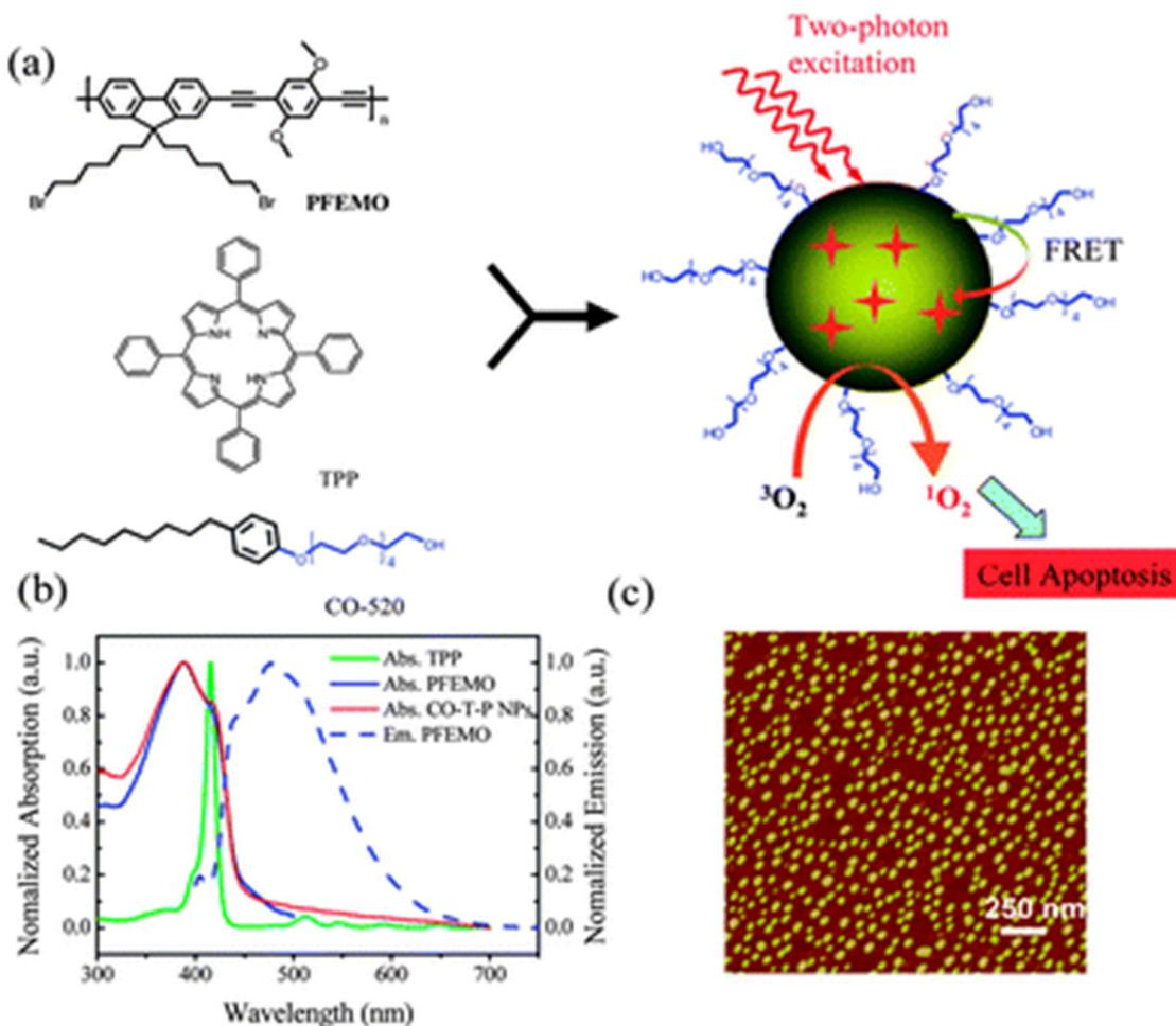
**Fig. 18** (a) Diagram showing the process of conjugated polymer nanoparticle formation for two-photon photodynamic therapy; (b) normalized absorption spectra of TPP, PFEMO and CO-T-P NPs (solid lines), and emission spectra of PFEMO (dashed line); (c) AFM imaging of CO-T-P NPs on a mica substation. Reproduced with permission.<sup>138</sup> Copyright 2011, Royal Society of Chemistry.
