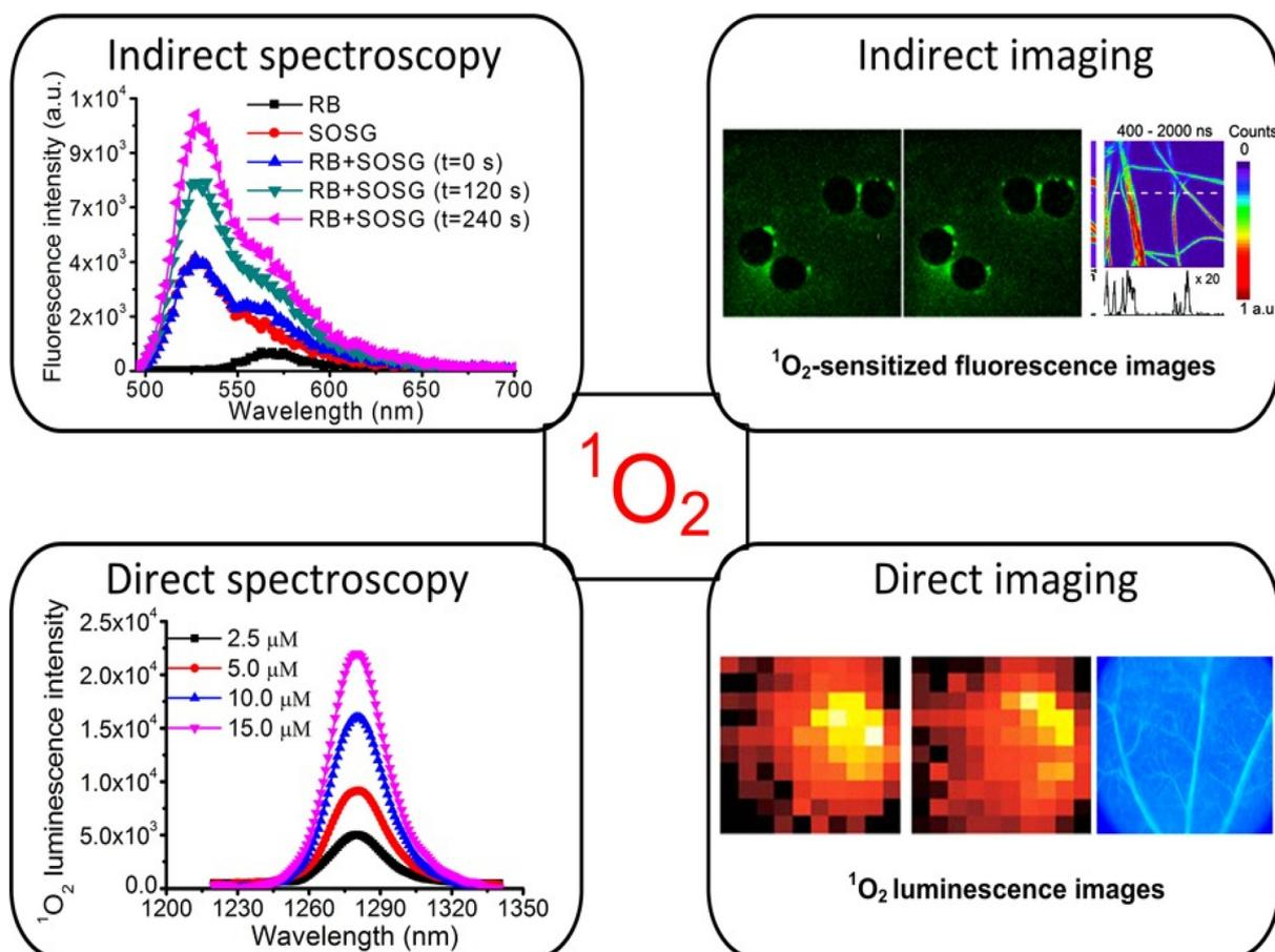
Fig. 4 Methods of  $^1\text{O}_2$  measurement using both direct and indirect detection.<sup>20</sup>
