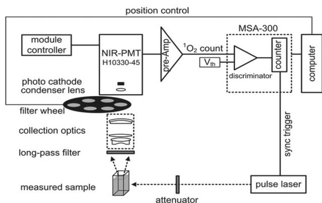
Fig. 5 Schematic diagram of the time- and wavelength-resolved  $^1\text{O}_2$  luminescence detection system.<sup>20</sup>
