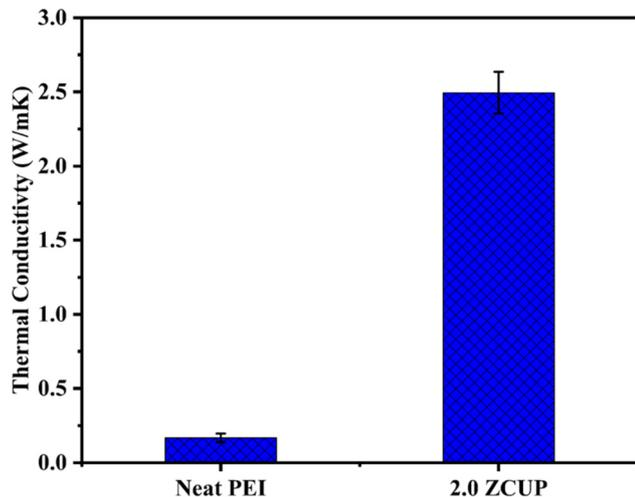
Fig. 10 Thermal conductivity of 2.0 ZCUP and PEI nanocomposites.
