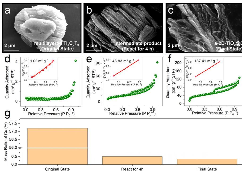
**Fig. 2** *Ex situ* investigations for analyzing samples at different reaction times. SEM images and nitrogen adsorption–desorption isotherms of (a and d) multilayered  $Ti_3C_2T_x$  (original state), (b and e) intermediate product (react for 4 h), and (c and f) a-2D- $TiO_2@C$  (final state). (g) Mass ratio of Cu in samples at different reaction times of the original state, sample after 4 h, and final state.
