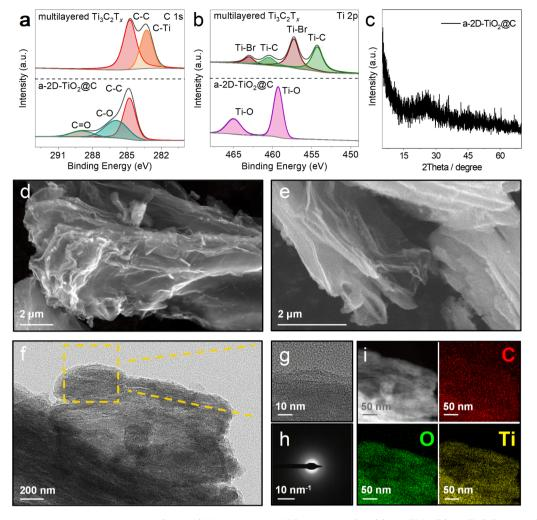
Fig. 3 Phase and morphological characterization. (a and b) High-resolution XPS spectra of C 1s (a) and Ti 2p (b) for  $Ti_3C_2T_x$  and a-2D-TiO<sub>2</sub>@C. (c) XRD pattern of a-2D-TiO<sub>2</sub>@C. (d and e) SEM images, (f) TEM image, (g) HRTEM image, (h) SAED pattern, and (i) scanning TEM image and the corresponding element mappings of a-2D-TiO<sub>2</sub>@C.
