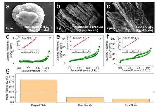
Fig. 2 Ex situ investigations for analyzing samples at different reaction times. SEM images and nitrogen adsorption-desorption isotherms of (a and d) multilayered Ti<sub>3</sub>C<sub>2</sub>T<sub>x</sub> (original state), (b and e) intermediate product (react for 4 h), and (c and f) a-2D-TiO<sub>2</sub>@C (final state). (g) Mass ratio of Cu in samples at different reaction times of the original state, sample after 4 h, and final state.
