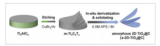
Fig. 1 Schematic of simultaneous derivatization and exfoliation of multilayered Ti<sub>3</sub>C<sub>2</sub>T<sub>x</sub> for the preparation of a-2D-TiO<sub>2</sub>@C.
