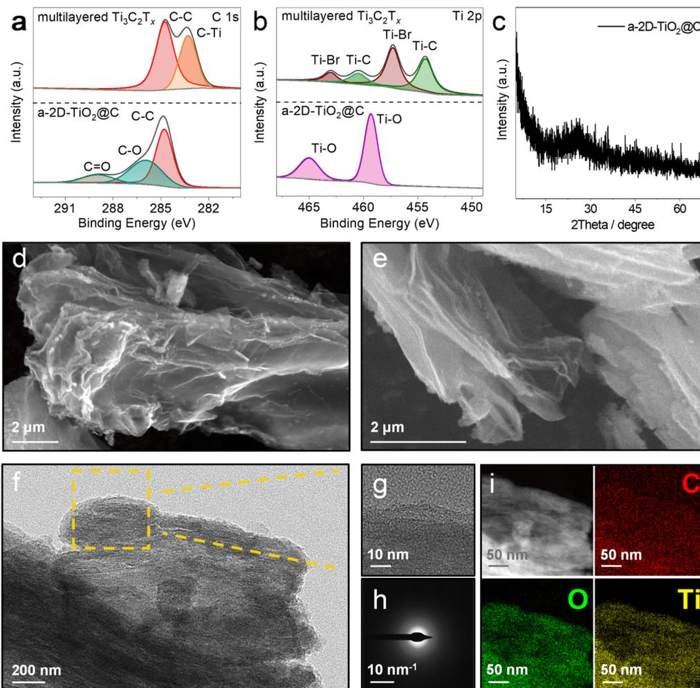
**Fig. 3** Phase and morphological characterization. (a and b) High-resolution XPS spectra of C 1s (a) and Ti 2p (b) for  $\text{Ti}_3\text{C}_2\text{T}_x$  and a-2D- $\text{TiO}_2@\text{C}$ . (c) XRD pattern of a-2D- $\text{TiO}_2@\text{C}$ . (d and e) SEM images, (f) TEM image, (g) HRTEM image, (h) SAED pattern, and (i) scanning TEM image and the corresponding element mappings of a-2D- $\text{TiO}_2@\text{C}$ .
