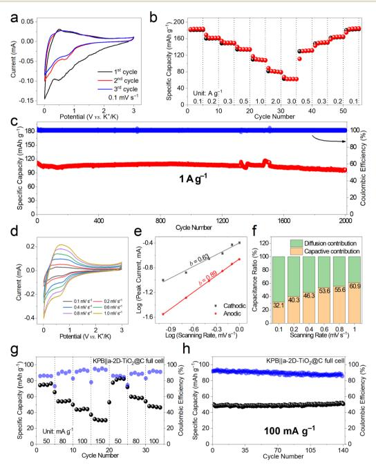
Fig. 4  $K^+$  storage behavior and performance. (a) The first three CV curves at 0.1 mV  $s^{-1}$ , (b) rate performance at 0.1–3.0 A  $g^{-1}$ , (c) long-term cyclability at 1 A q<sup>-1</sup>, (d) CV curves at 0.1-1.0 mV s<sup>-1</sup>, (e) b values of cathodic and anodic peaks, and (f) pseudocapacitance proportion of a-2D-TiO<sub>2</sub>@C. (g) Rate performance (50–100 mA g<sup>-1</sup>) and (h) cycling stability of KPB||a-2D-TiO<sub>2</sub>@C full cells.
