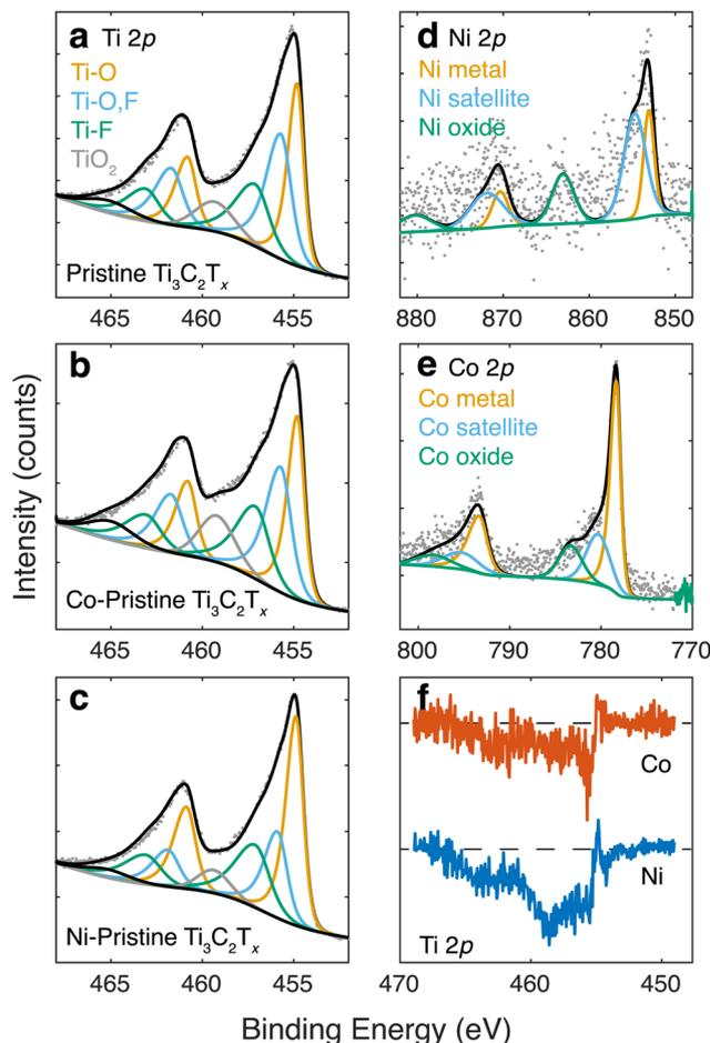
**Fig. 4** X-ray photoelectron spectroscopy (XPS) of the (a–c) Ti 2*p* core-level from (a) pristine  $\text{Ti}_3\text{C}_2\text{T}_x$  MXene, and after (b) Co and (c) Ni metal incorporation. Corresponding (d) Ni 2*p* and (e) Co 2*p* spectra. (f) Difference spectra, obtained by subtracting the metal-incorporated spectra from the pristine MXene spectra, for the Ti 2*p* core-level, indicating slight oxidation of the MXene during metal incorporation.
