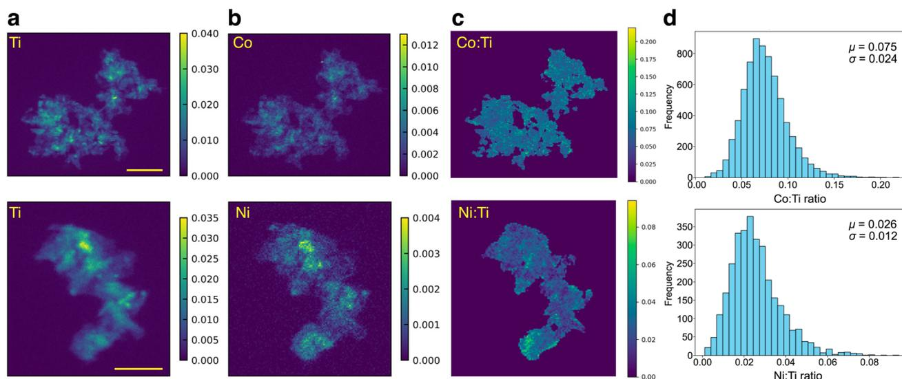
**Fig. 3** X-ray fluorescence (XRF) mapping of MXene flakes drop-cast onto Si substrates. (a) Ti XRF map, (b) XRF map of the incorporated metal, and (c) intensity ratio of the incorporated metal and Ti. Scale bars are 2  $\mu\text{m}$ . (d) Histograms showing the distribution of Co vs. Ti and Ni vs. Ti from the concentration values within each pixel in the XRF maps.
