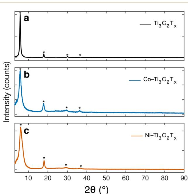
**Fig. 2** X-ray diffraction (XRD) patterns of (a) pristine  $\text{Ti}_3\text{C}_2\text{T}_x$  MXene, and after (b) Co and (c) Ni metal incorporation. The 00 $l$  peaks marked with asterisks (\*) indicate the out-of-plane alignment of the MXene sheets in the free-standing films.
