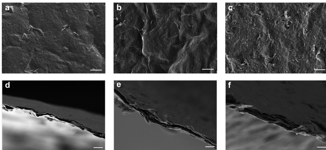
**Fig. 1** Scanning electron microscopy (SEM) images of (a and d) pristine and (b and e) Co and (c and f) Ni incorporated  $\text{Ti}_3\text{C}_2\text{T}_x$  MXene free-standing films showing the (top) surface and (bottom) cross-section. Scale bars are 5  $\mu\text{m}$  for (a–c) and 2  $\mu\text{m}$  for (d–f).
