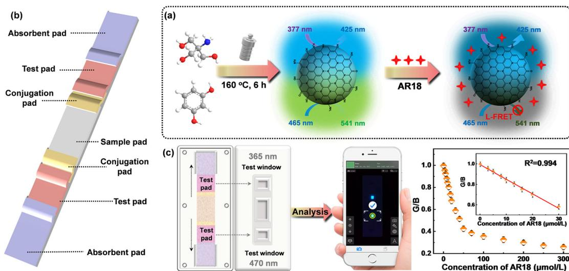
**Fig. 1** Schematic representation of the preparation process and applications of N-CDs. (a) Schematic diagram of the preparation process of N-CDs. (b) Structure diagram of the LFTS. (c) Hardware design of a smartphone fluorometric sensing platform for AR18 detection using a smartphone app.
