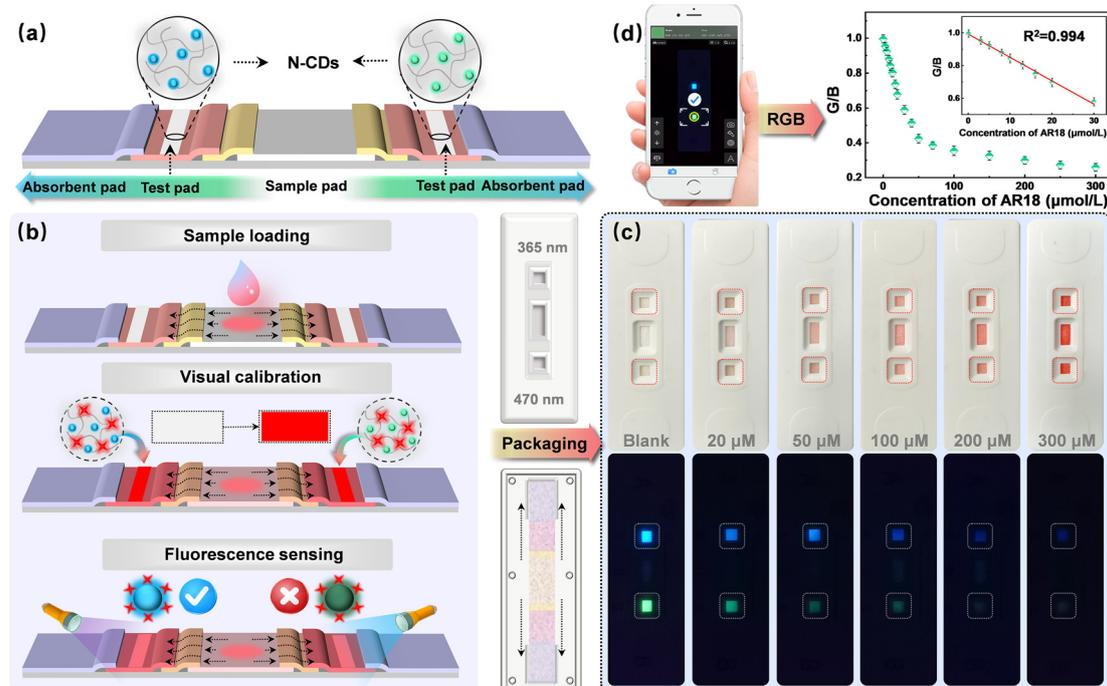
**Fig. 5** (a) Hardware design of the LFTS. (b) Operation diagram illustrating the functioning of the LFTS. (c) Images of the sensing platform utilizing the LFTS with varying concentrations of AR18. (d) Correlation between the ratio value of  $G/B$  and the concentration of AR18.
