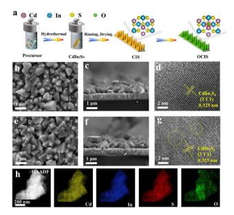
Fig. 1 (a) The synthetic schematic for the OCIS photoanode. The topview SEM images of (b) CIS, and (e) OCIS. The cross-sectional SEM images of (c) CIS and (f) OCIS. HRTEM images of (d) CIS and (g) OCIS. (h) EDS mapping of OCIS.
