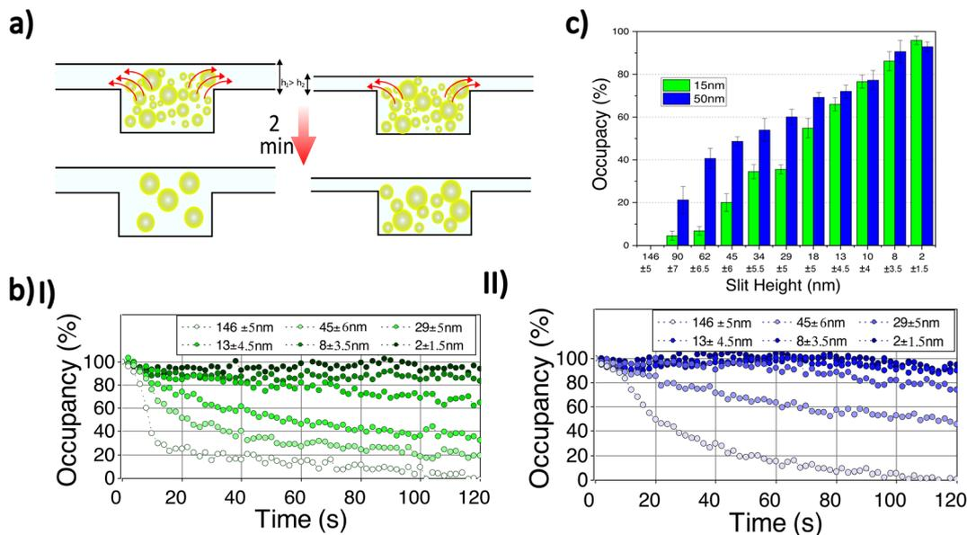
**Fig. 4** (a) Schematic images of particle retention at two slit heights. (b) Time-dependence of percent occupancy for (b-I) 15 nm and (b-II) 50 nm particles retained in nanocavities for a range of slit heights. Percent occupancy refers to percentage of particles that remain in cavity at a given time (as inferred from particle fluorescence). (c) Percent occupancy for 15 and 50 nm nanoparticles retained in cavities for different slit heights after 2 min have elapsed.
