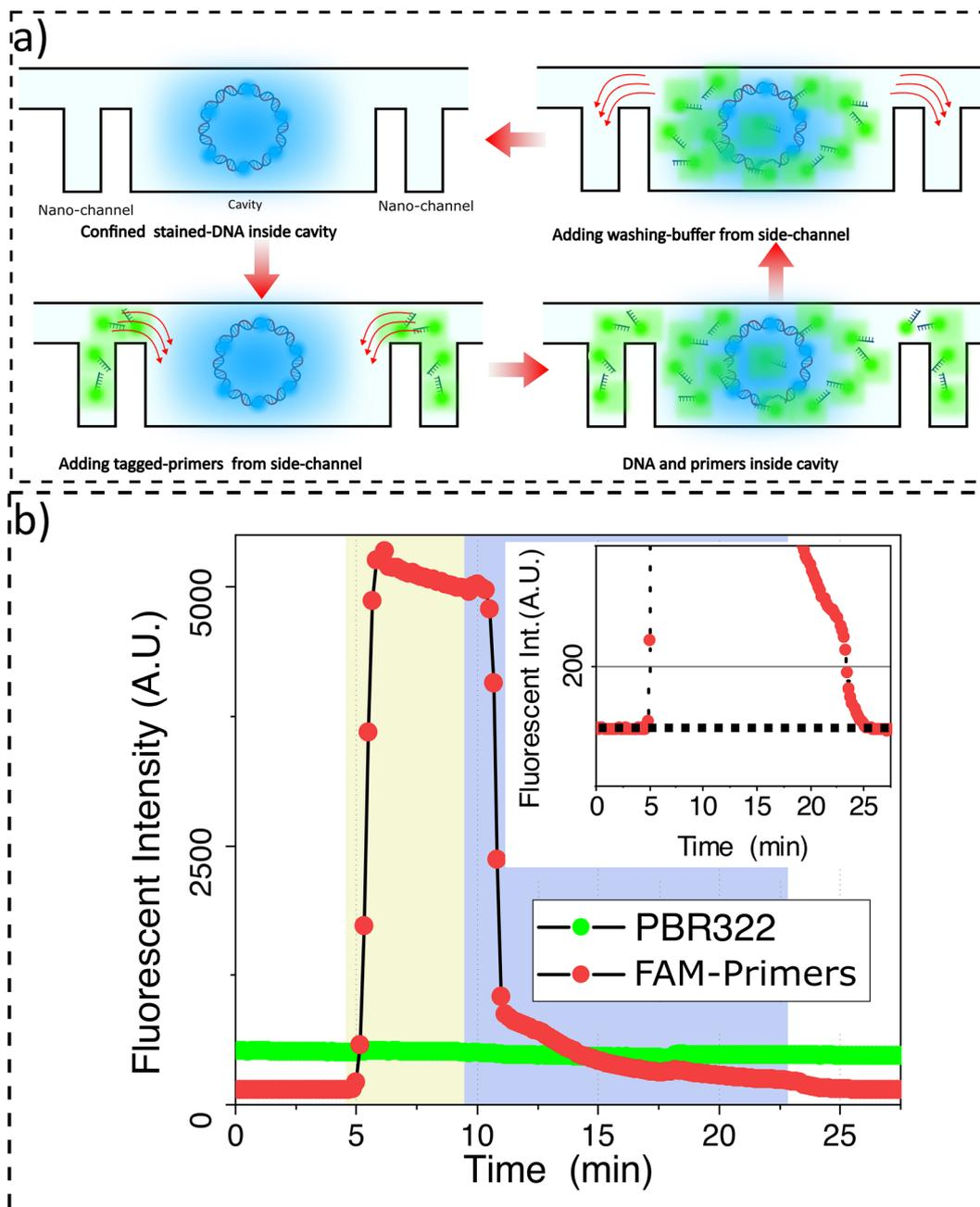
**Fig. 3** (a) Schematic showing target molecule retention inside cavities while small nucleic acids are loaded and then washed away from the cavities. (b) Retention of YOYO-3 labelled-pBR322 plasmid vectors in nanocavities during the introduction of FAM-tagged primers (20 bp). The inset shows the relative intensity, the intensity normalized to the intensity before loading primers; this reaches zero when the cavities are completely empty of primers.
