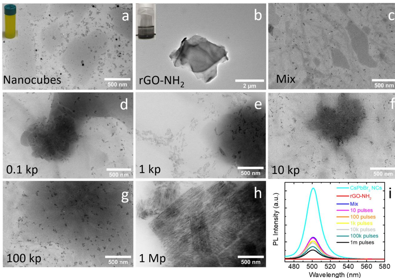
**Fig. 1** Transmission electron microscopy (TEM) images of the metal halide perovskite nanocrystals (a), the amine-functionalized rGO sheets (b), a mixture of the two materials in toluene prior to irradiation (c), the conjugated dispersions after irradiation with 100–1 million pulses (d–h), and the corresponding PL curves (i). Insets in (a) and (b): digital photographs of the perovskite nanocrystals' and rGO sheets' toluene-based colloidal dispersions.
