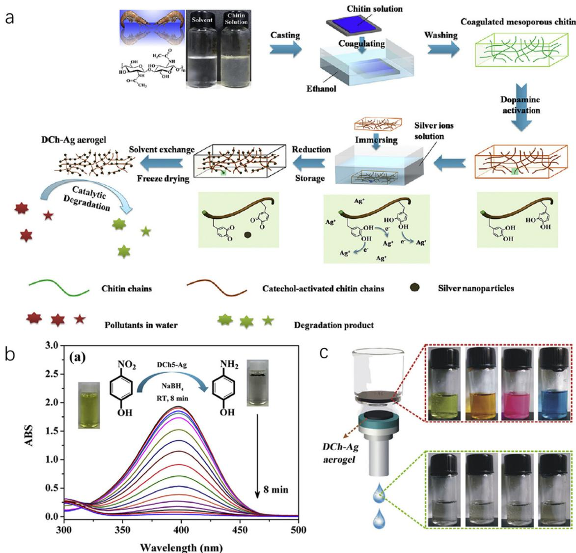
**Fig. 10** (a) Illustration of the fabrication of the ChNC-Ag aerogel. (b) Catalytic evaluation of ChNC-Ag NP aerogels with a typical UV-vis spectra of the conversion reaction. The inset photographs show the color change from yellow (before) to colorless (after). (c) ChNC-Ag aerogels as filtration membranes to remove organic pollutants, where four colored organic dyes become colorless after the filtration process. Reproduced with permission.<sup>142</sup> Copyright 2017, Elsevier Inc.
