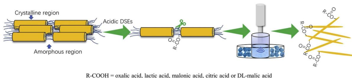
Fig. 5 Illustration of nanochitin synthesis using organic acid DESs. Reproduced with permission.<sup>81</sup> Copyright 2020, Elsevier Ltd.
