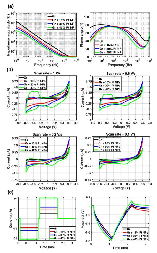
Fig. 4 (a) Average EIS results of 7 samples per graphene without Pt NPs and 5 samples per each set of NP surface densities, (b) CV curves of the median sample of each category of graphene without and with NPs with different surface densities, (c) the median of the maximum-amplitude current pulse applied to 5 electrodes per each category of different NP densities with the corresponding VT measurement.
