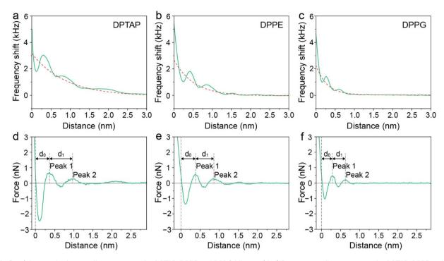
Fig. 4 (a-c) Averaged Δf versus distance curves for DPTAP, DPPE and DPPG bilayers. (d-f) Force versus distance curves for DPTAP, DPPE and DPPG bilayers converted from  $\Delta f$  curves
